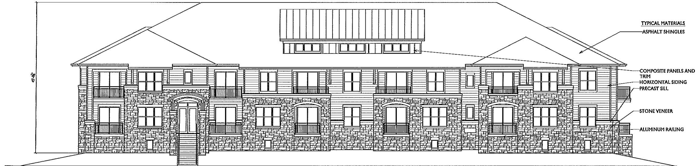
1 WEST ELEVATION - BUILDING I 6 SCALE: 1/8"=1'-0"
