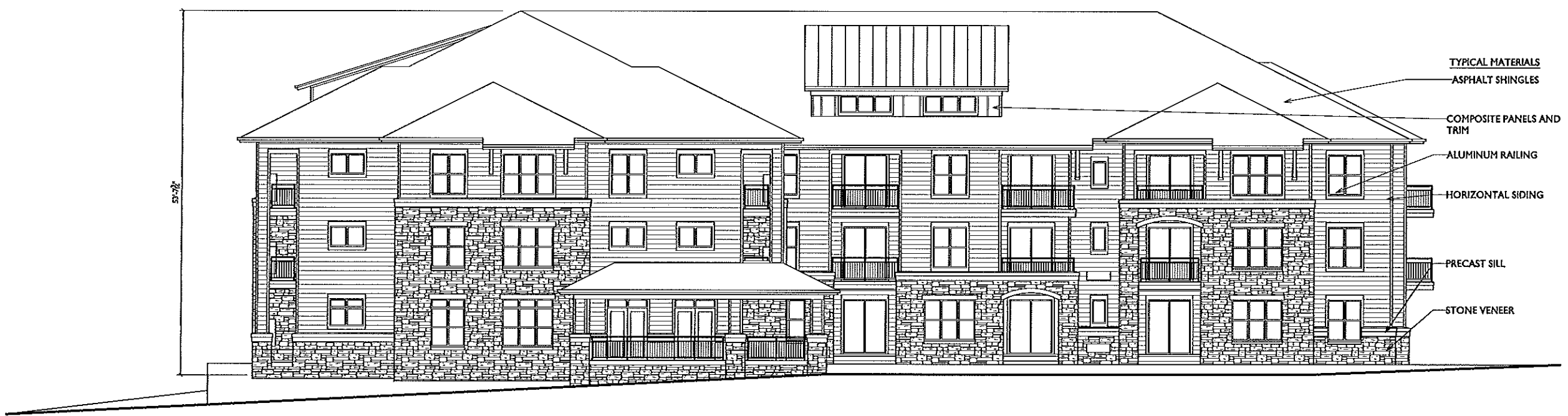
1 SOUTH ELEVATION - BUILDING 3 15 SCALE: 1/8"=1'-0"
