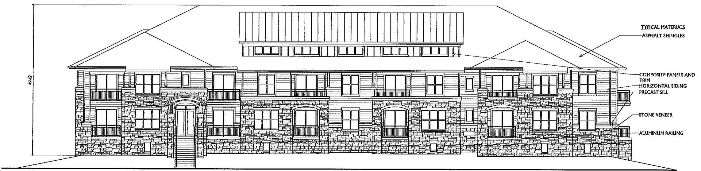
1 WEST ELEVATION - BUILDING I SCALE: 1/8"=1'-0"
