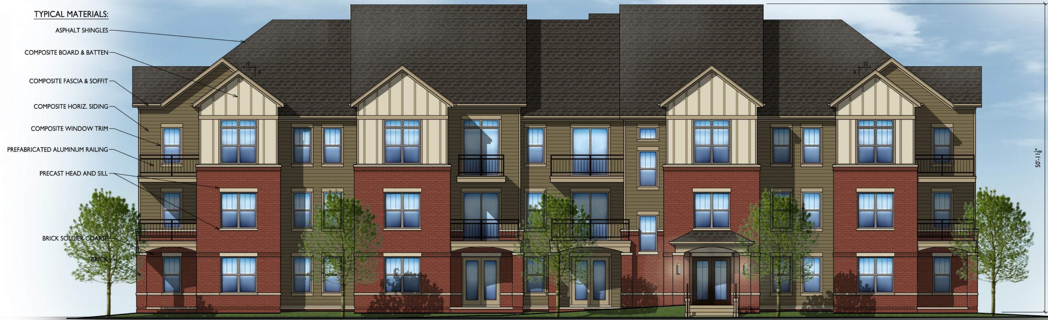
BUILDING #3 WEST ELEVATION 1 A-2.2 1/8"=1'-0"
