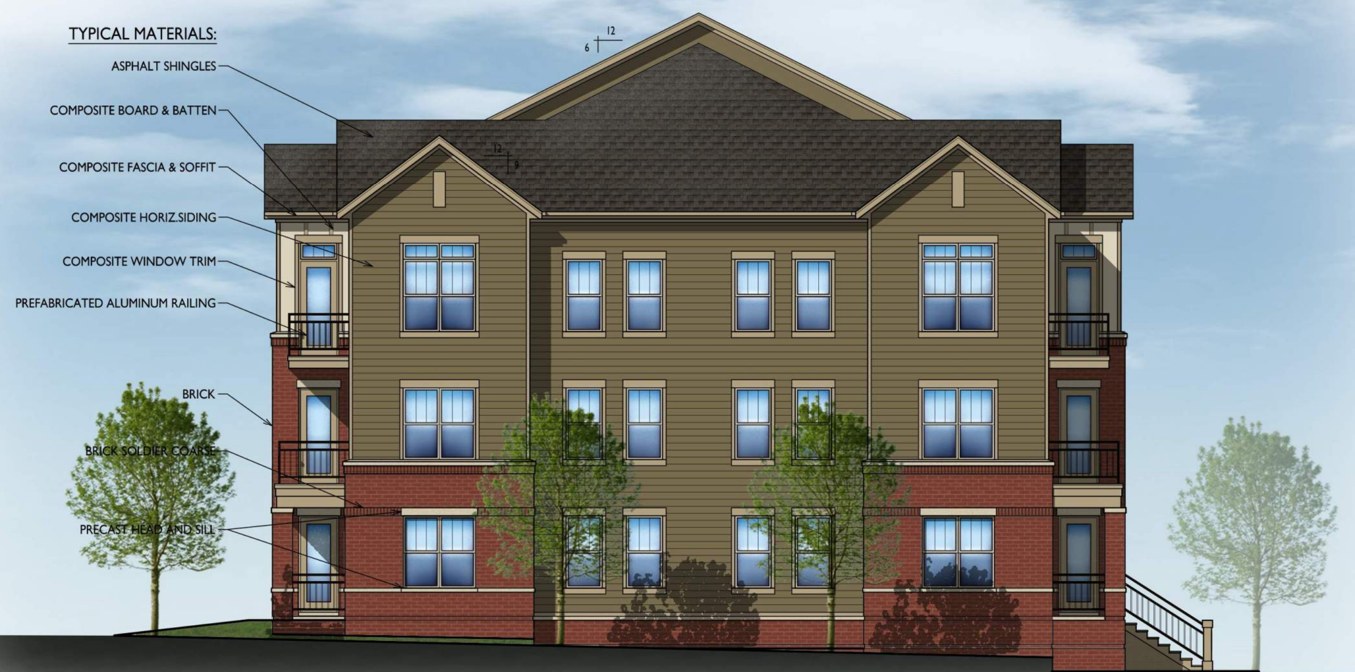
BUILDING #3 SOUTH ELEVATION 2 A-2.1 1/8"=1'-0"
