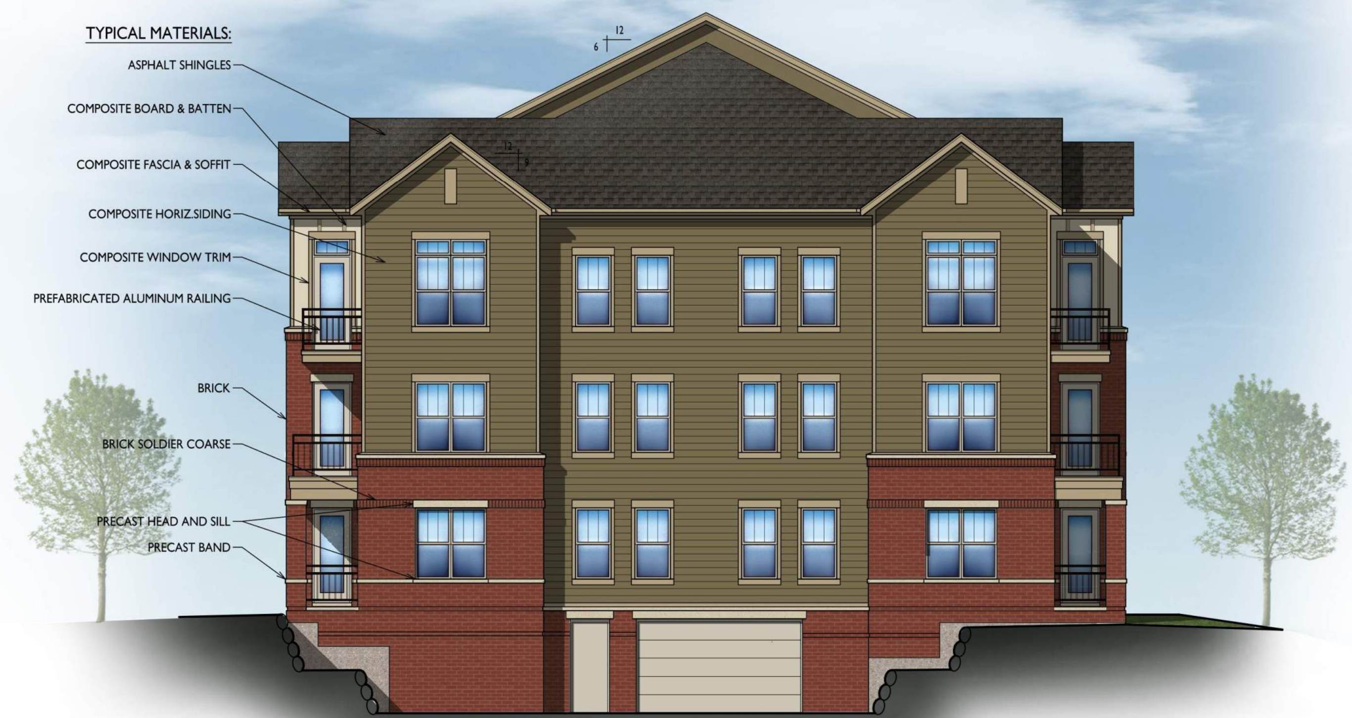
BUILDING #2 SOUTH ELEVATION 2 A-2.2 1/8"=1'-0"
