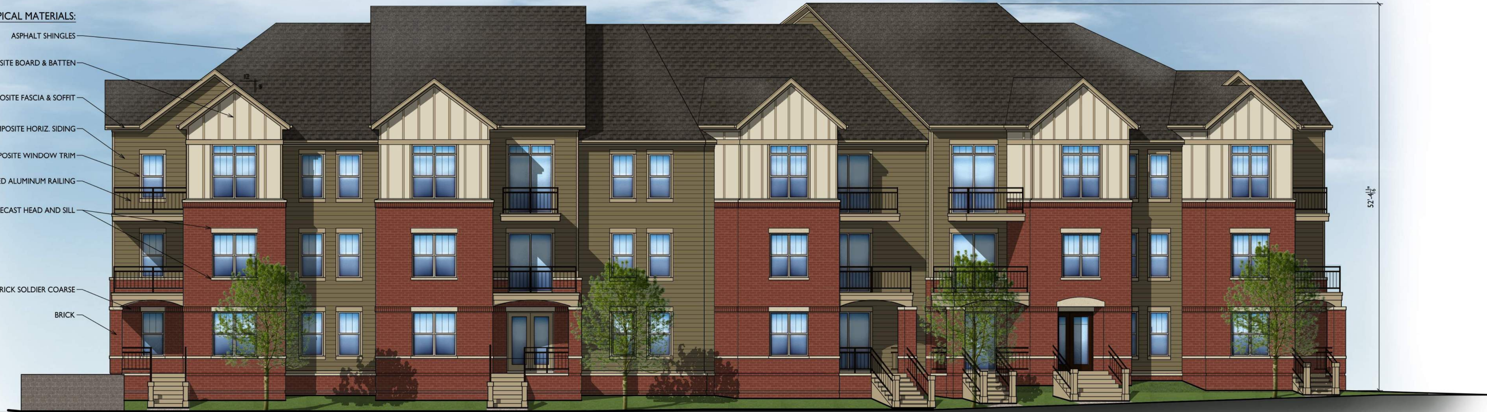
BUILDING #1 EAST ELEVATION ALONG METRO TERRACE 1 A-2.1 1/8"=1'-0"
