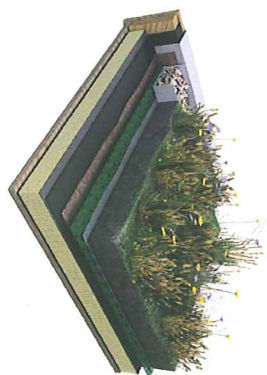
THE GREEN ROOF WILL UTILIZE A SEMI-INTENSIVE GREEN ROOF SECTION. SEMI-INTENSIVE REFERS TO THE SOIL MEDIUM - TYPICALLY 6" - 12" - WHICH ALLOWS FOR VARIED NATIVE PERENNIALS AND EVEN SMALL SHRUBS. THE ILLUSTRATIONS ABOVE, CREATED BY ALEX JOHNSON, SHOW A TYPICAL SEMI-INTENSIVE GREEN SECTION.
