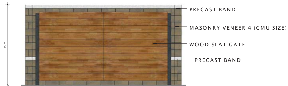
11 TRASH ENCLOSURE GATE ELEVATION 3/8" = 1'-0"
