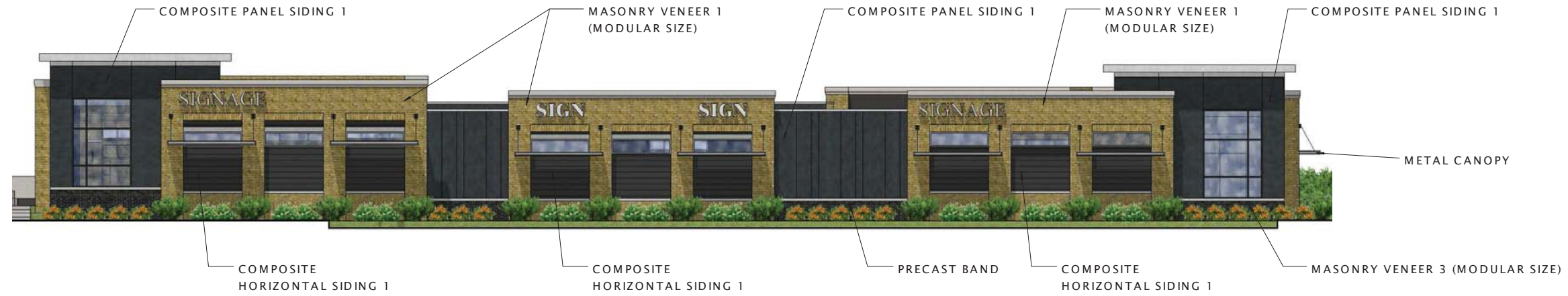
⑥ B5 SOUTH ELEVATION 1/8" = 1'-0"
