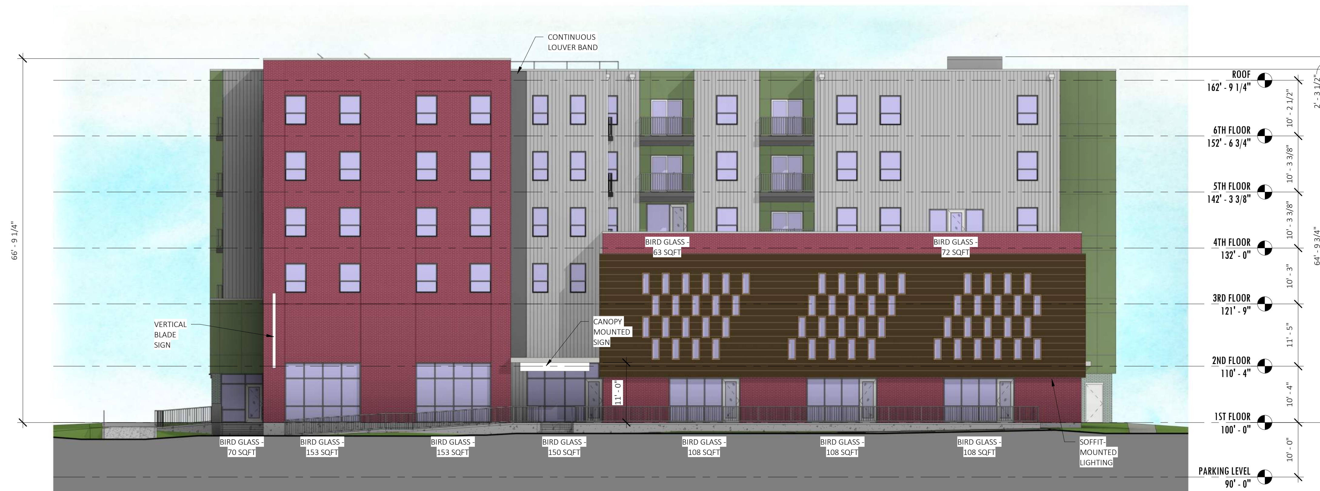
2 WEST ELEVATION - 18% GLAZING SCALE: 3/32" = 1'-0"
