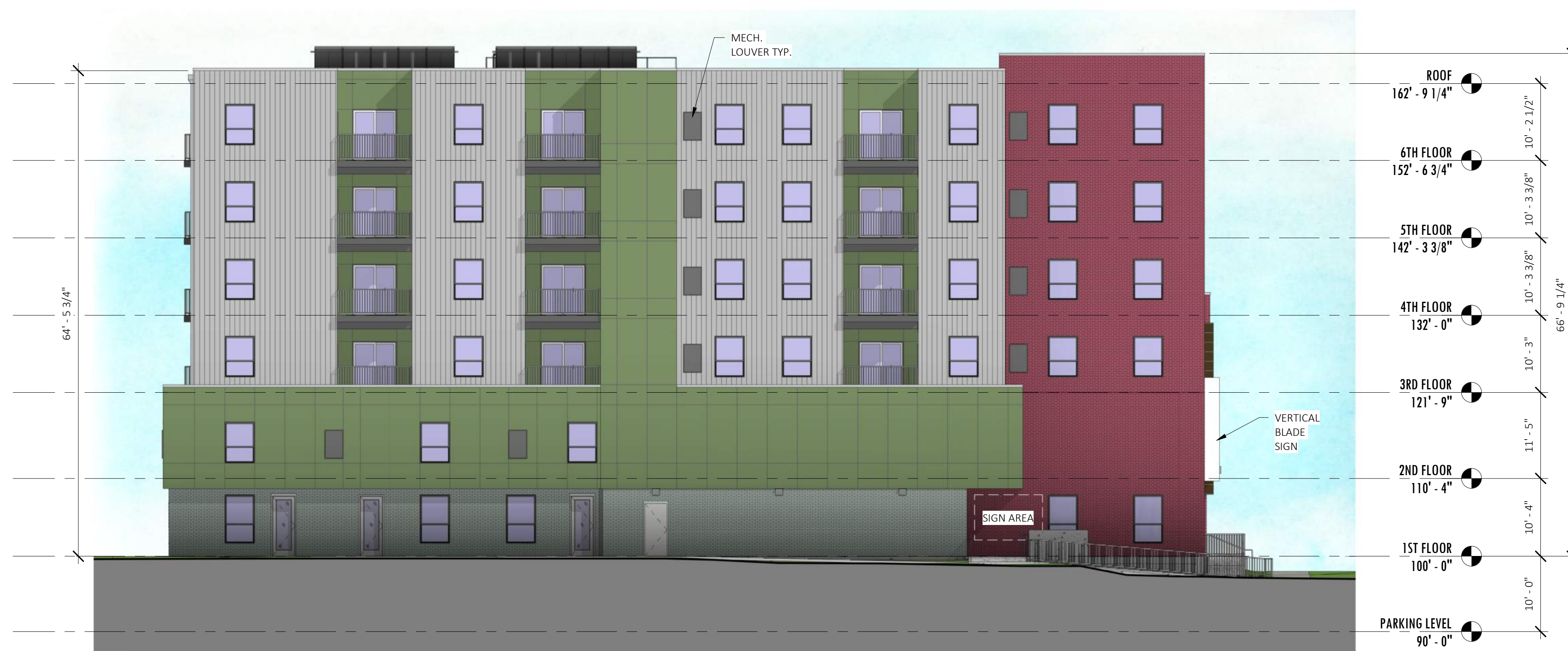
1 NORTH ELEVATION - 15% GLAZING SCALE: 3/32" = 1'-0"
