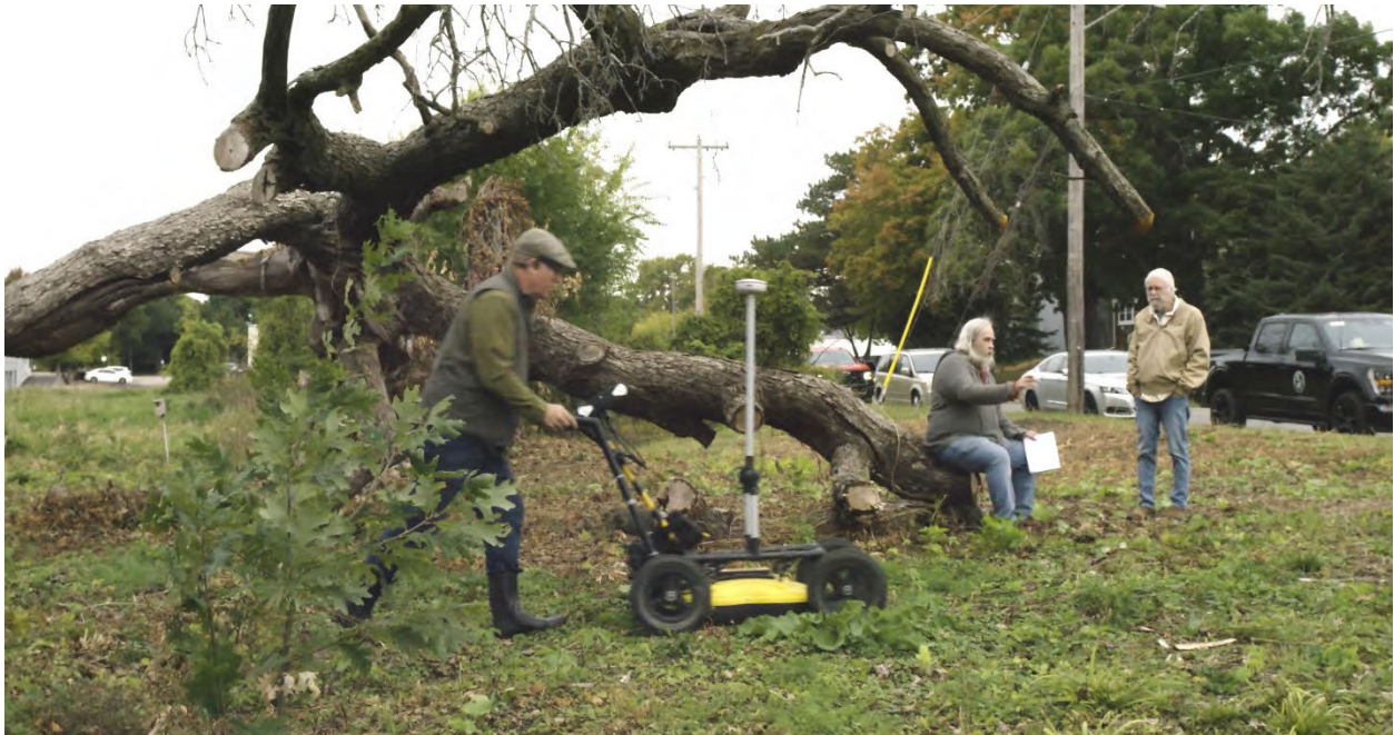
Figure 8: Ben Hanson pushes the GPR past the fallen marker tree (see Figure 3). A monitor just above his hands is displaying raw data.
