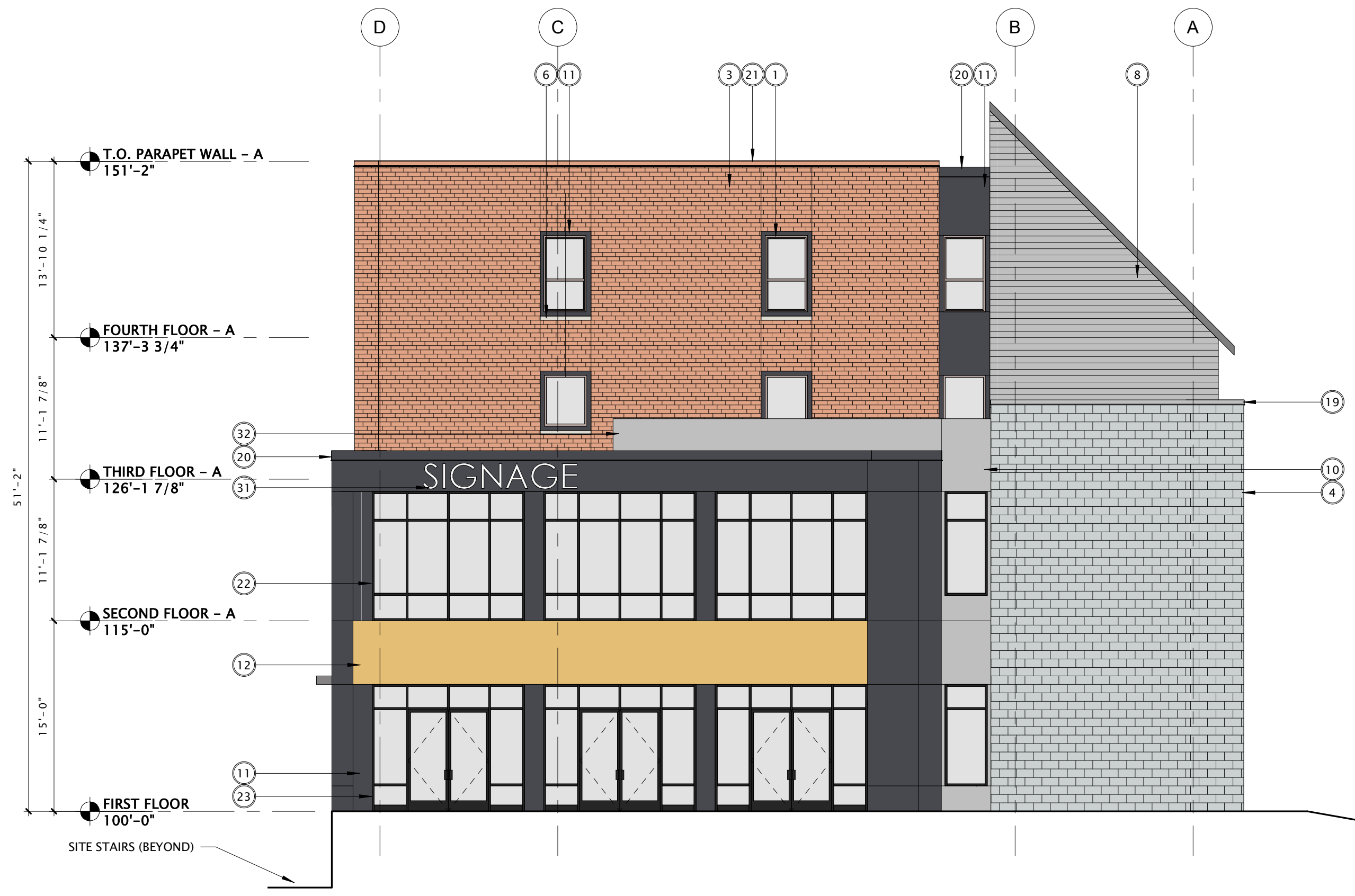
13 BUILDING 'A' - NORTH ELEVATION 1/8" = 1'-0"
