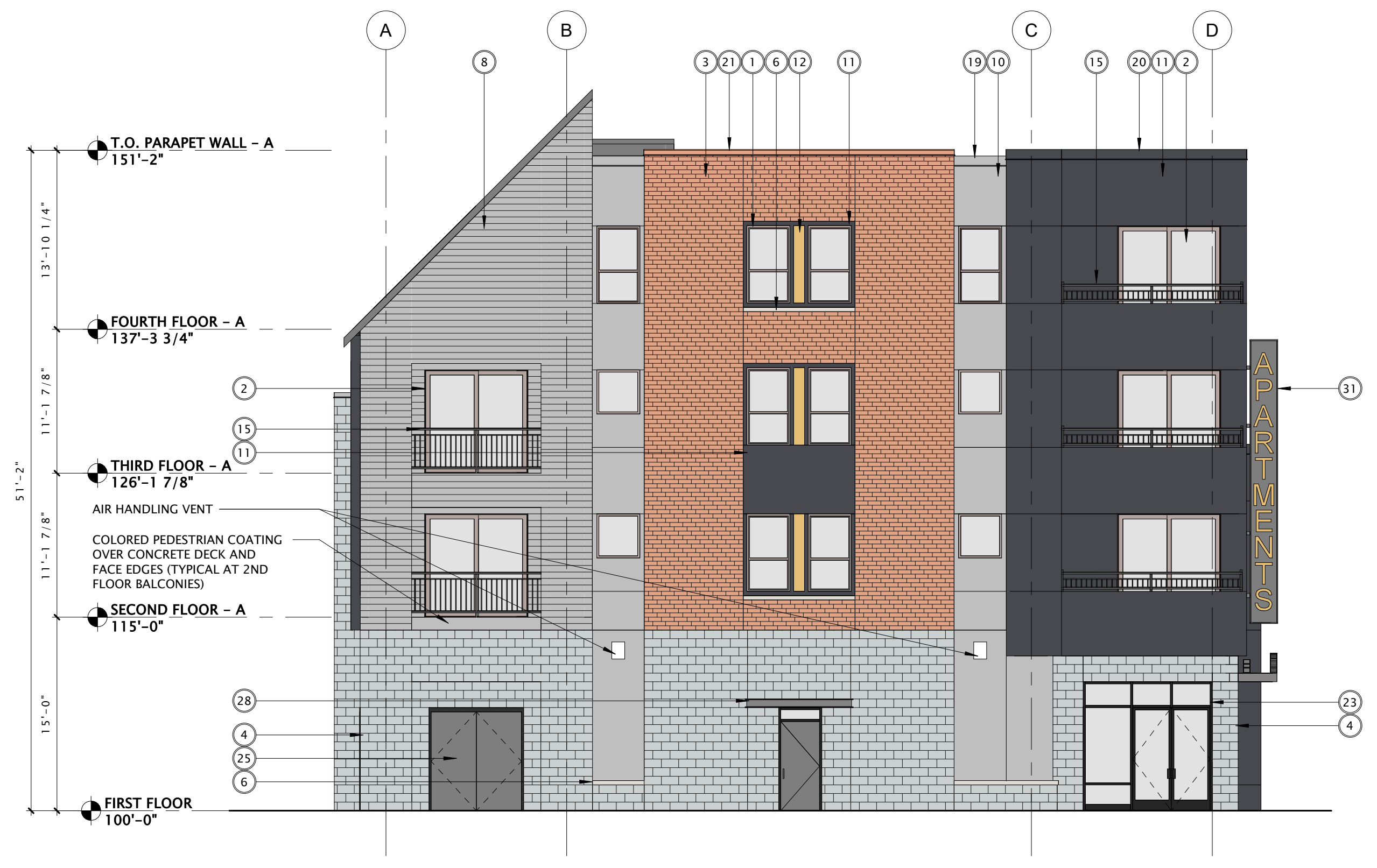
18 BUILDING 'A' - SOUTH ELEVATION 1/8" = 1'-0"
