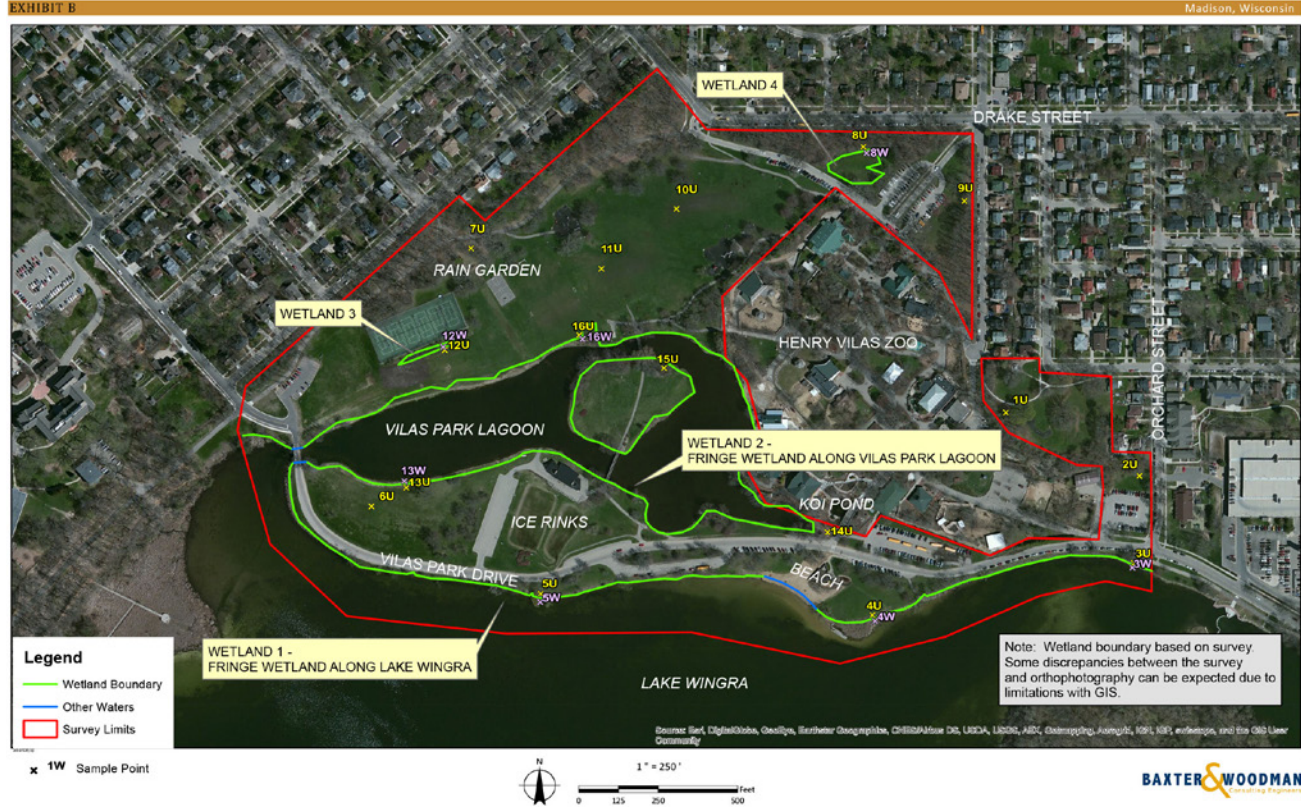
Figure 5.146. Wetland Boundary Map (Wetland Delineation of Vilas Park - Baxter and Woodman Consulting Engineers, 2016)
