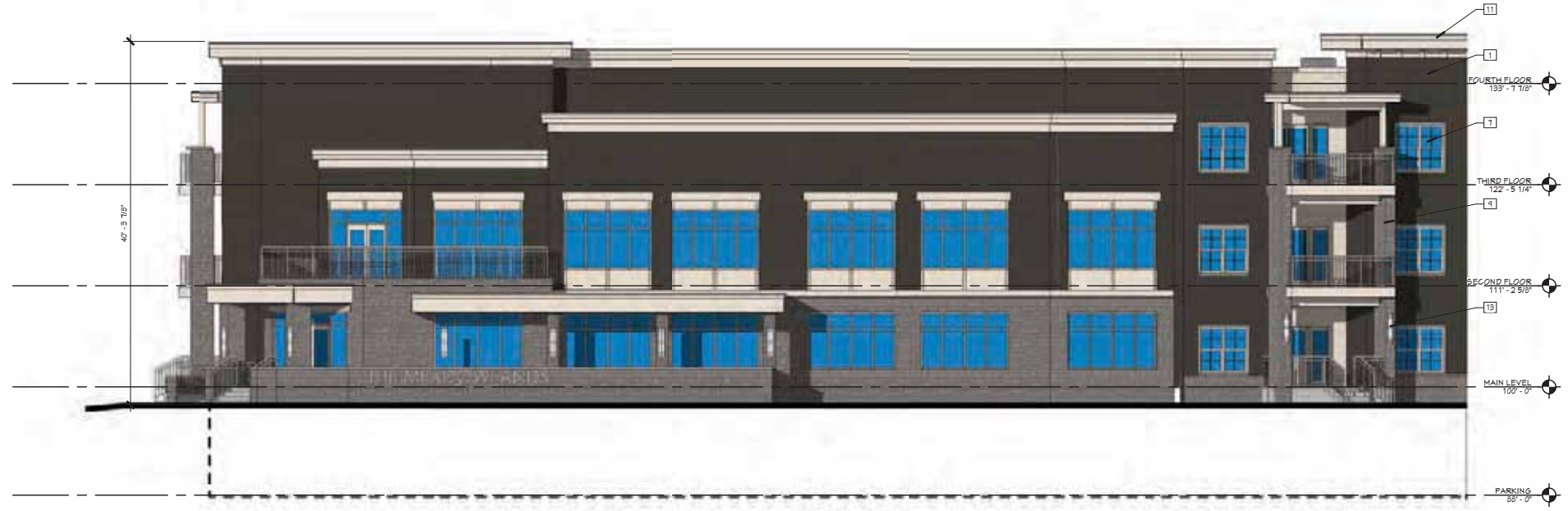
2 A4.8 BUILDING 4 - EAST ELEVATION 1/8" = 1'-0"
