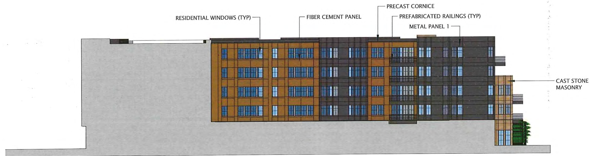
② SOUTH COURTYARD ELEVATION 1/32" = 1'-0"
