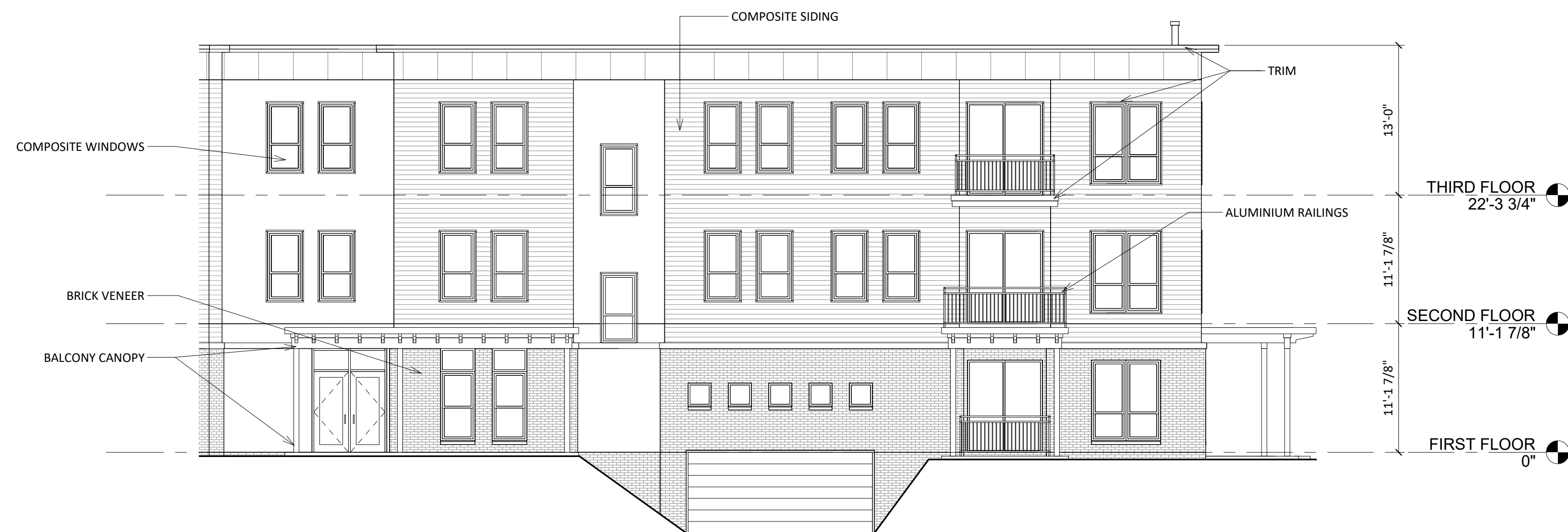
4 SOUTH WEST ELEVATION 1/8" = 1'-0"
