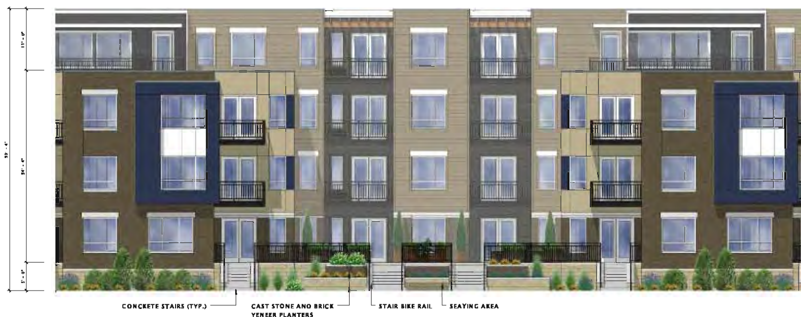
③ Mifflin Street Courtyard Enlarged Elevation 1/8" = 1'-0"
