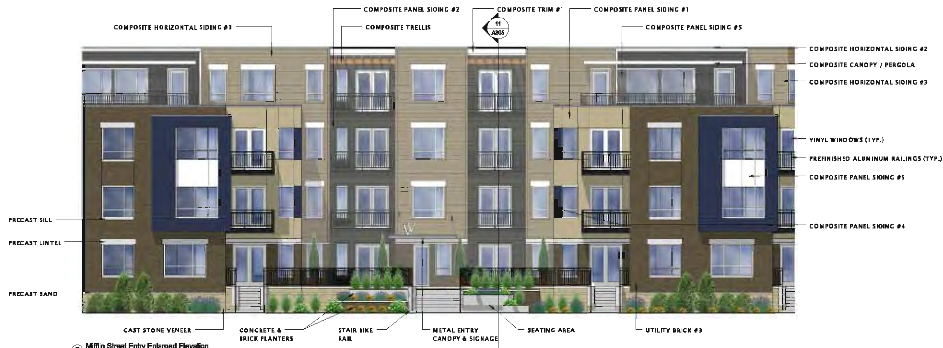
② Mifflin Street Entry Enlarged Elevation 1/8" = 1'-0"
