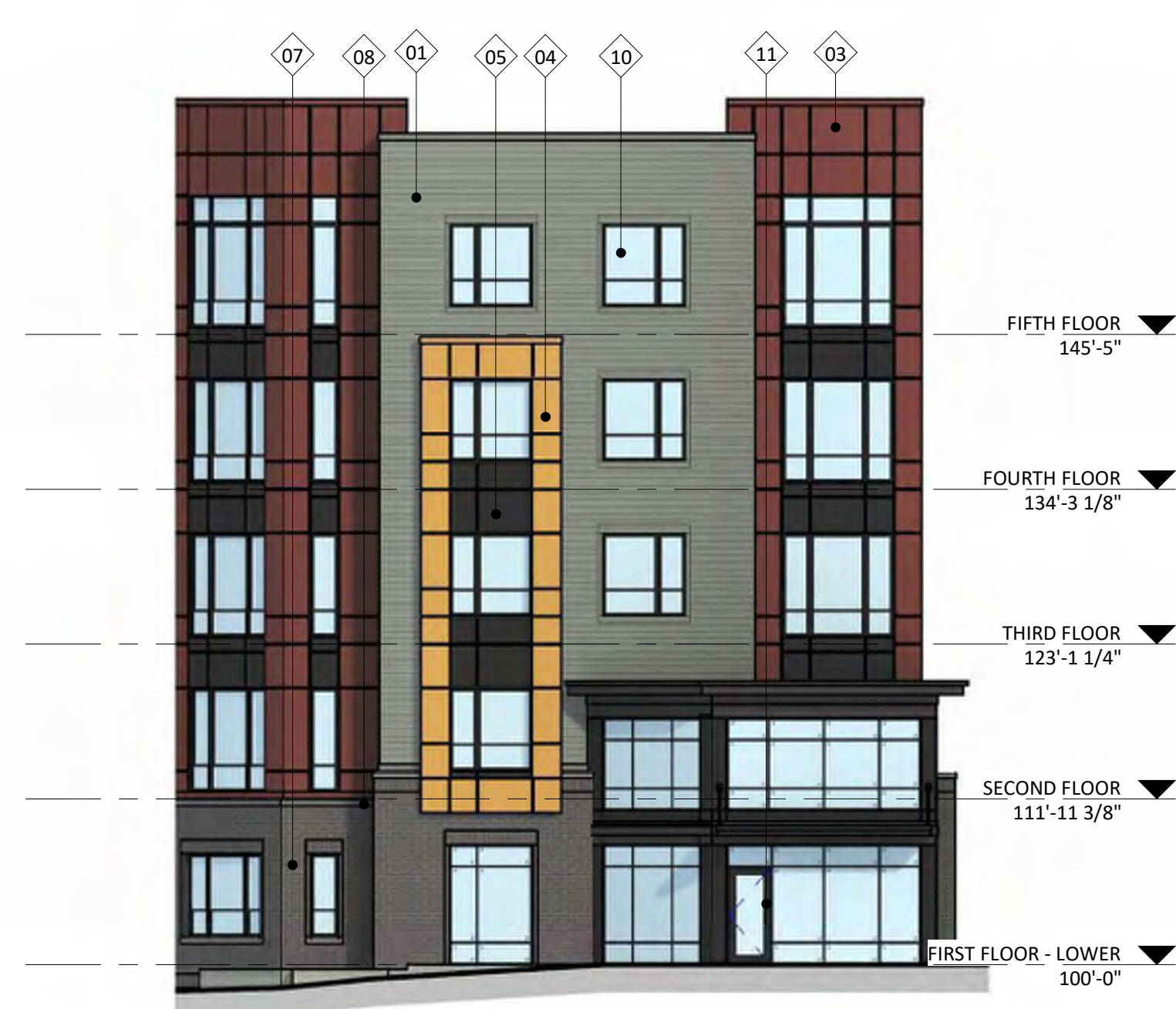
NORTHEAST ELEVATION AT CORNER
