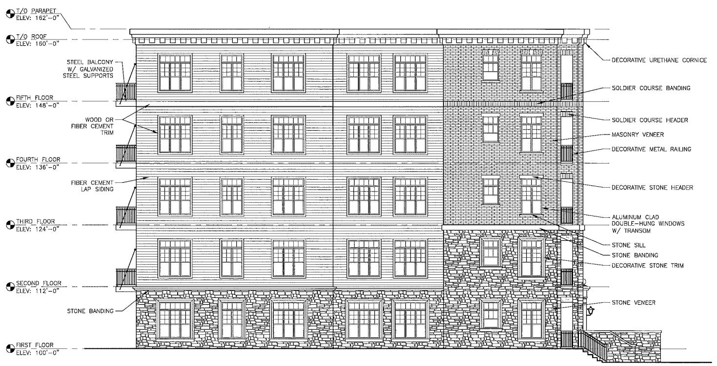
2 SIDE ELEVATION - 123 W. GILMAN SCALE: 1/8"=1'-0"
