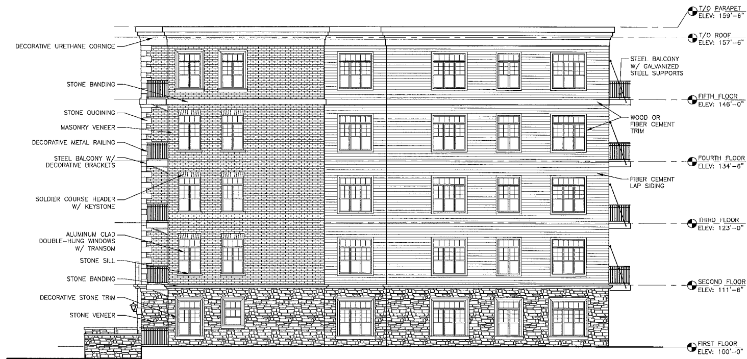
1 SIDE ELEVATION - 121 W. GILMAN SCALE: 1/8"=1'-0"
