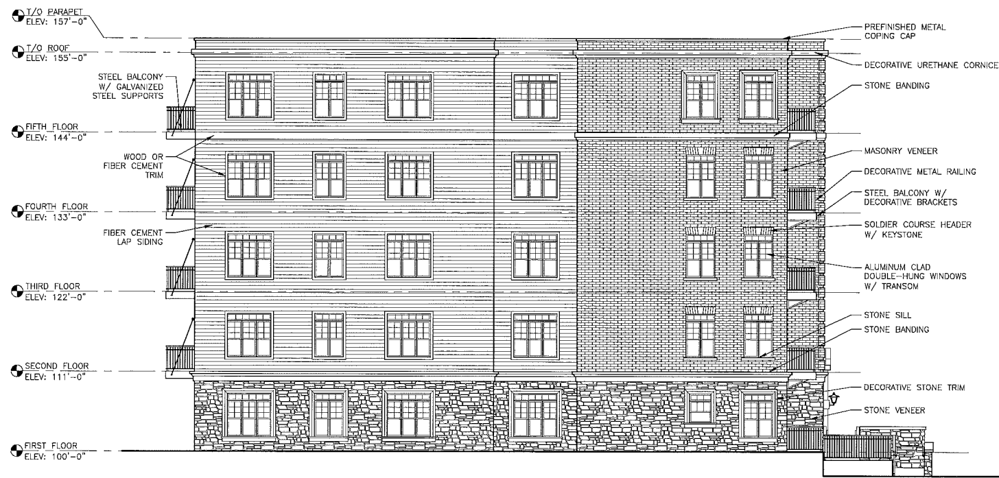
2 SIDE ELEVATION - 127 W. GILMAN SCALE: 1/8"=1'-0"
