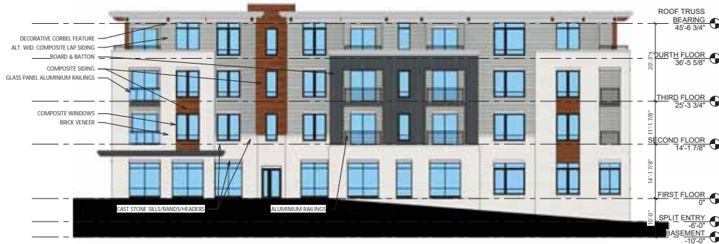
2 A-2.4 BLDG #5 - WEST ELEVATION COLORED 3/32" = 1'-0"
