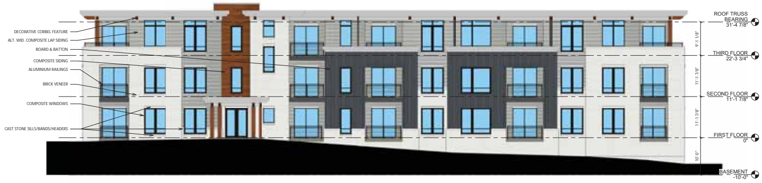
1 A-2.3 1/8" = 1'-0" BLDG #4 - WEST ELEVATION COLORED
