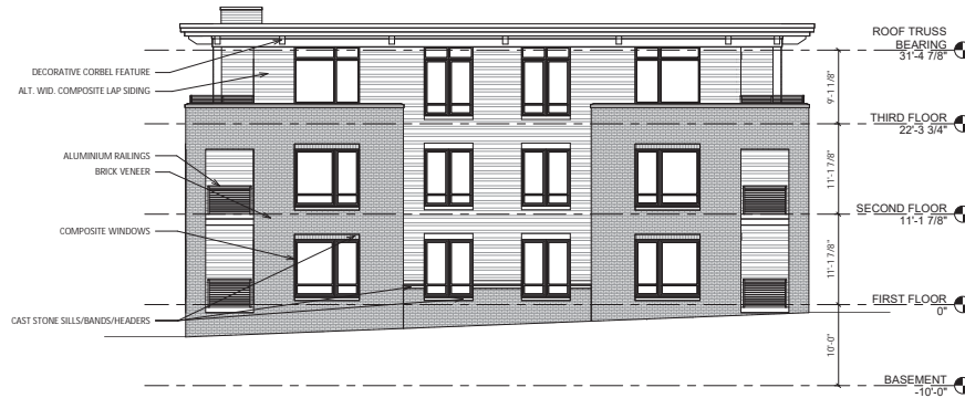
1 BLDG #7 - NORTH ELEVATION A-2.2 1/8" = 1'-0"
