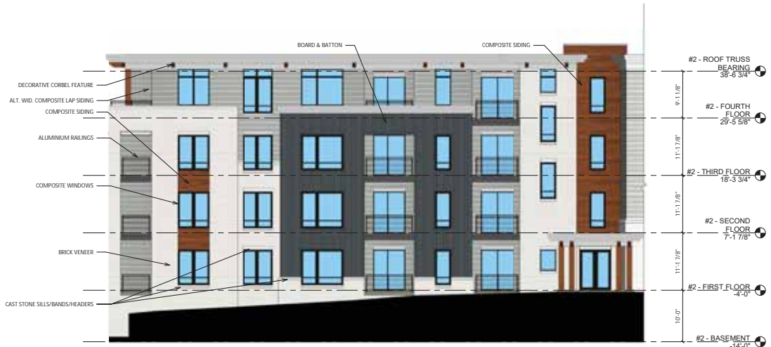
2 BLDG #2 - NORTH ELEVATION - ANGLE COLORED A-2.4 1/8" = 1'-0"
