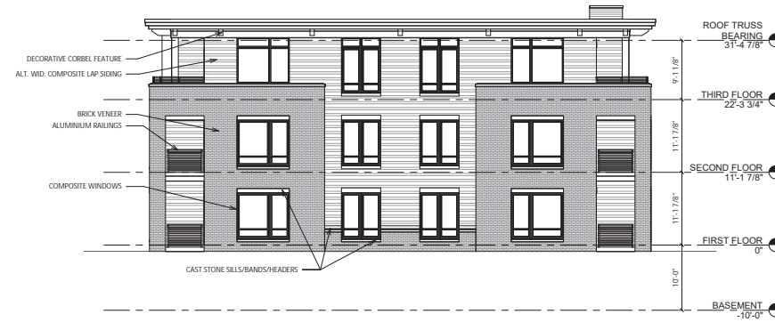
1 BLDG #4 - NORTH ELEVATION A-2.2 1/8" = 1'-0"
