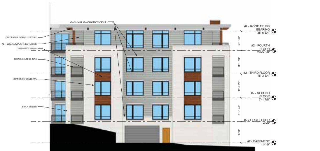
4 BLDG #2 - SOUTH ELEVATION - ANGLE COLORED A-2.4 1/8" = 1'-0"
