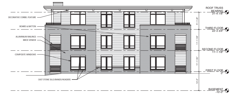
1 BLDG #6 - NORTH ELEVATION A-2.2 1/8" = 1'-0"
