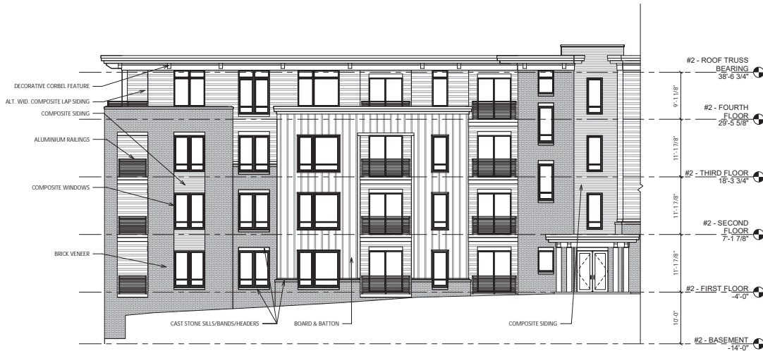
2 A-2.1 BLDG #2 - North Elevation-Angle 1/8" = 1'-0"
