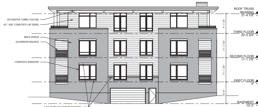
2 BLDG #4 - SOUTH ELEVATION A-2.2 1/8" = 1'-0"
