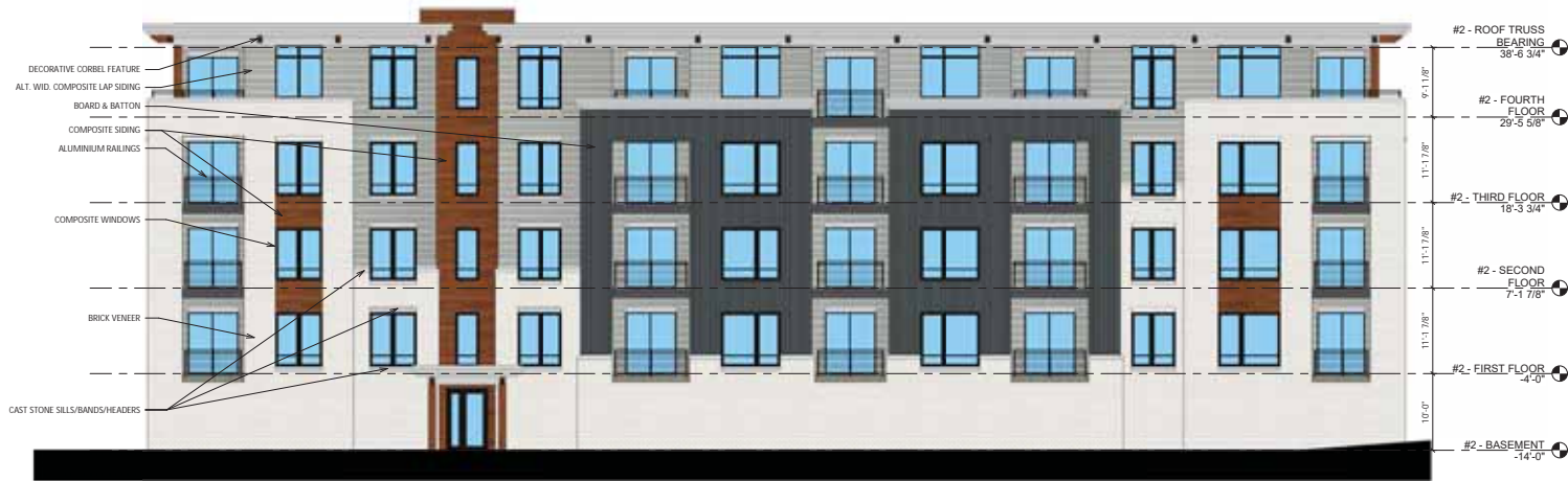
1 A-2.3 BLDG #2 - EAST ELEVATION - ANGLE COLORED 1/8" = 1'-0"
