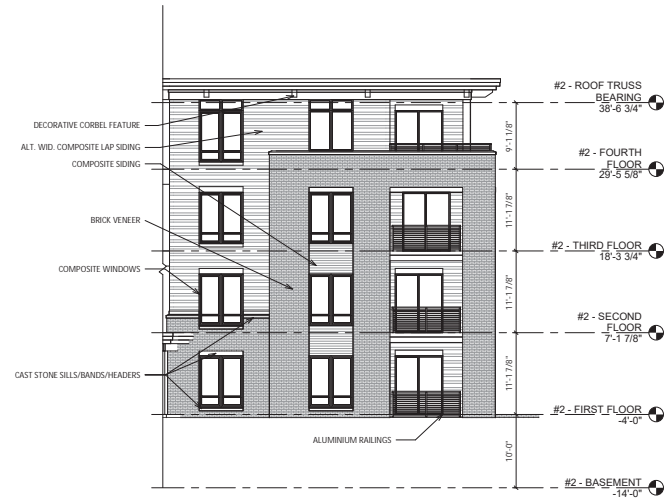
1 A-2.1 BLDG #2 - North Elevation 1/8" = 1'-0"
