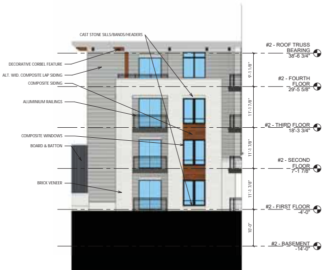
3 BLDG #2 - SOUTH ELEVATION COLORED A-2.4 1/8" = 1'-0"
