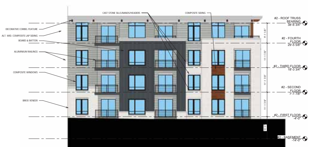
3 A-2.3 BLDG #2 - WEST ELEVATION - ANGLE COLORED 1/8" = 1'-0"
