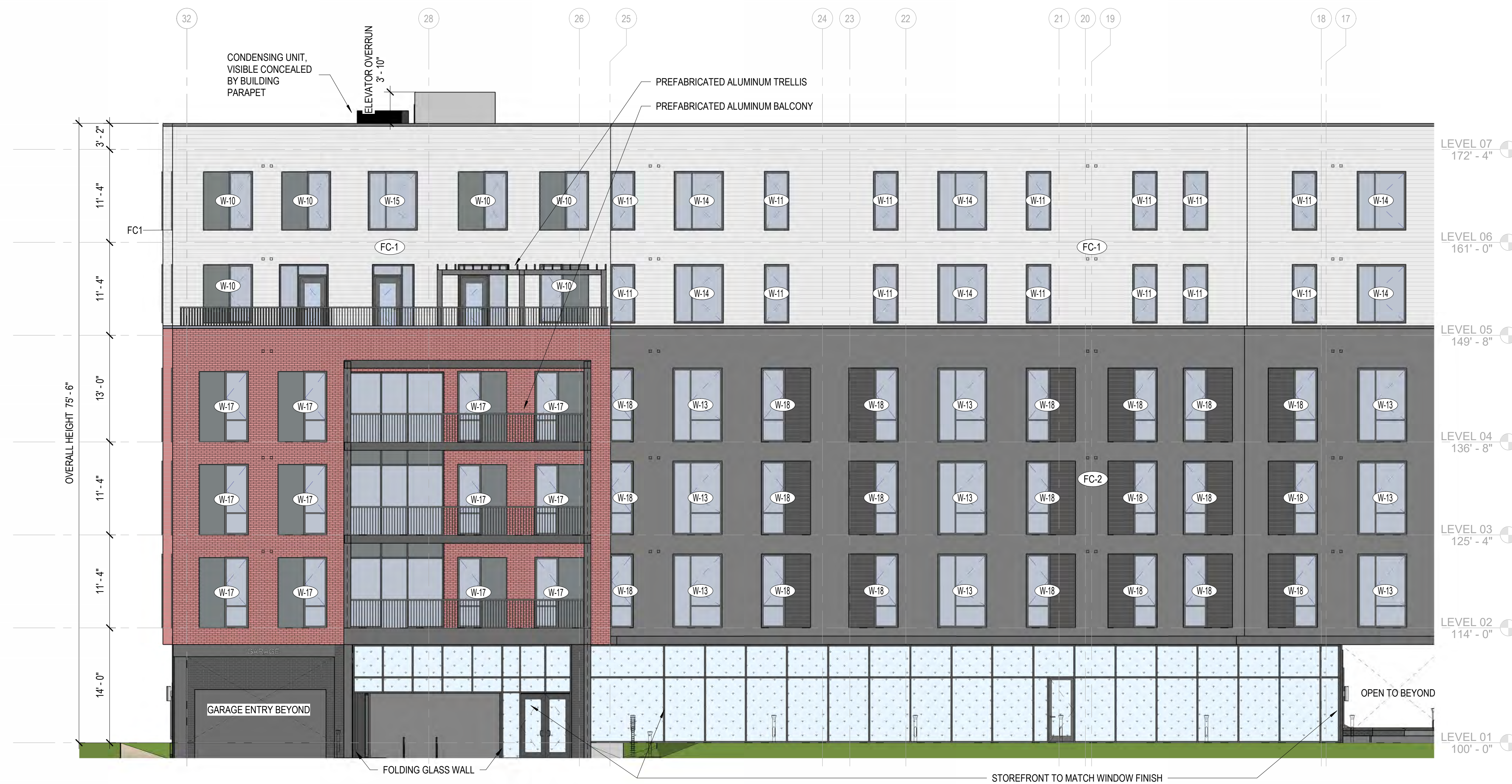
E3 ENLARGED ELEVATION - NORTH - AREA A A6.102 1/8" = 1'-0"
