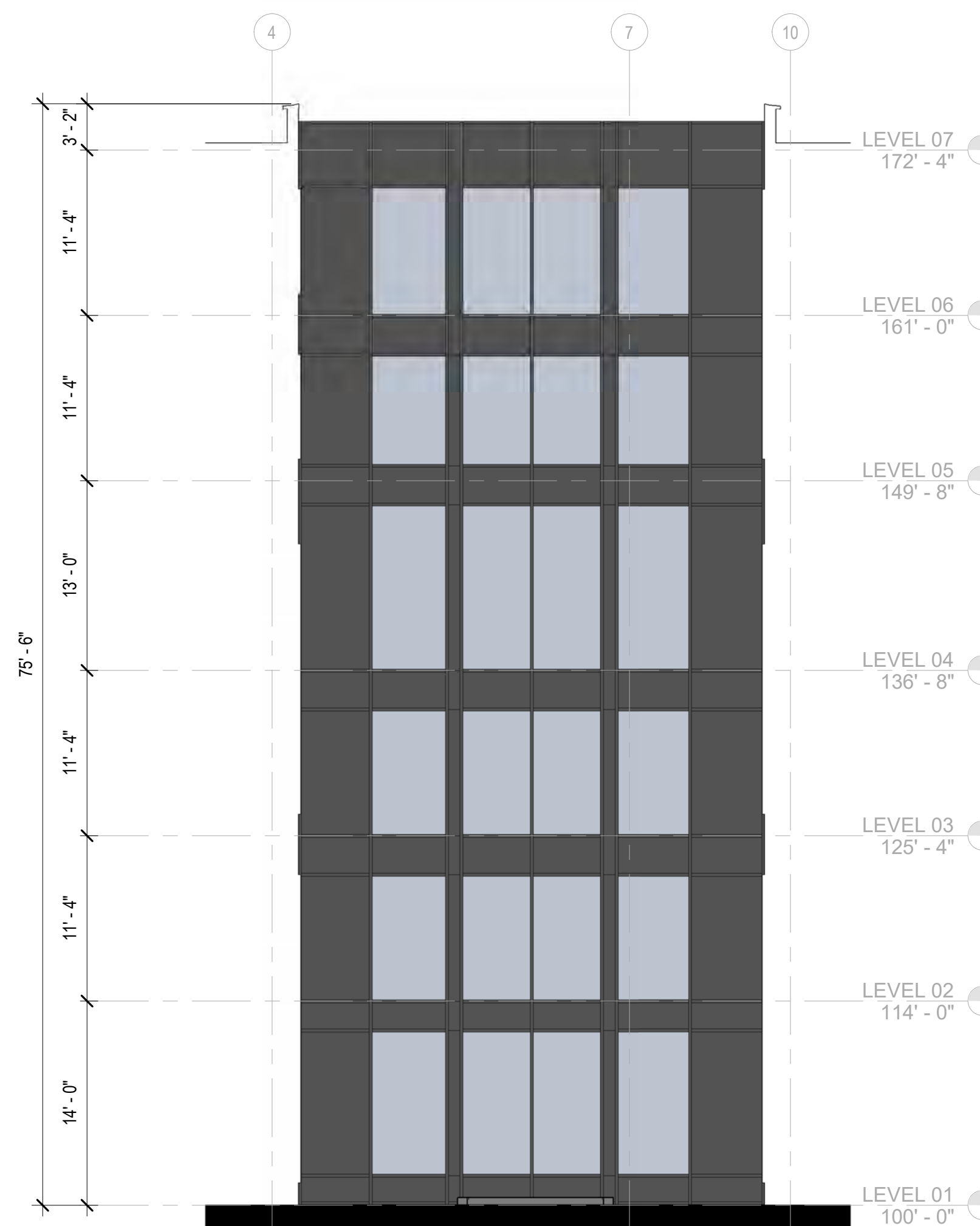
C1 ENLARGED ELEVATION - NORTH - ENCLOSED A6.107 1/8" = 1'-0"
