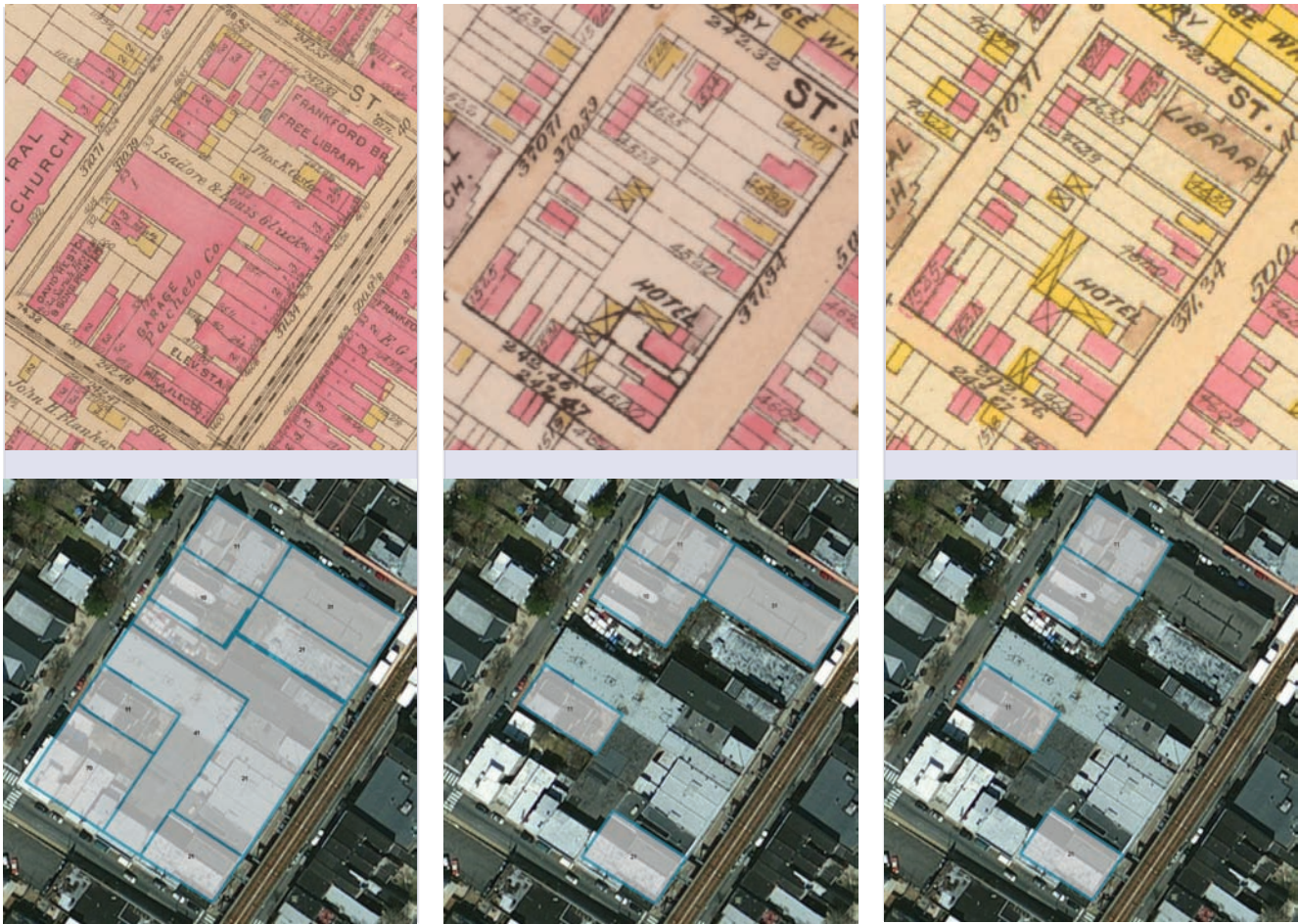
3.6-3.8 These historic maps and corresponding GIS polygons show the origins of the built environment, from 1929 (left) to 1910 to 1895. Following the classification of contemporary groupings (Figures 3.2-3.5), surveyors use historic maps to determine when each grouping appeared in its current form.
