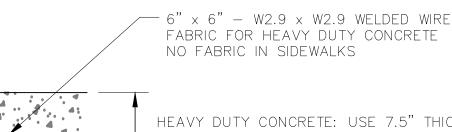
HEAVY DUTY CONCRETE: USE 7.5" THICK FOR LOADING DOCK AND DROP OFF LANE. EDGES SHALL BE THICKENED TO 12".
