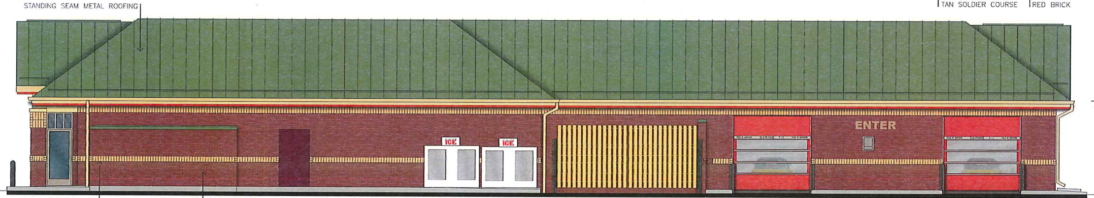
STANDING SEAM METAL ROOFING | RED FASCIA | WHITE FASCIA TAN SOLDIER COURSE | RED BRICK
