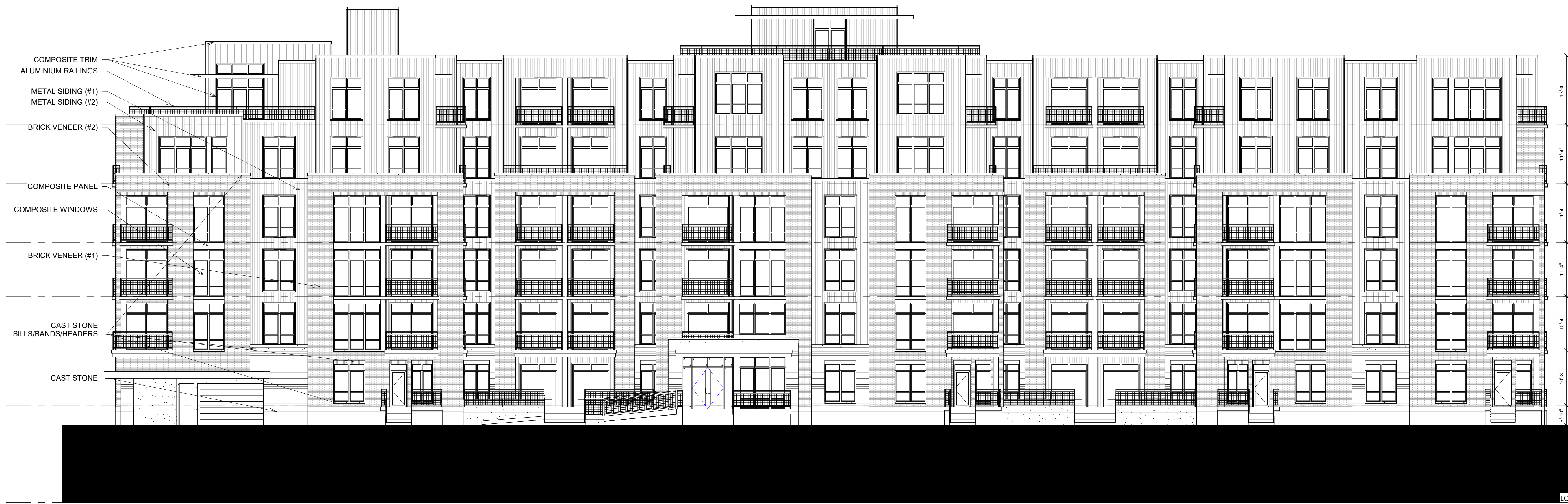
1 ELEVATION - NORTH A-2.1 3/32" = 1'-0"
