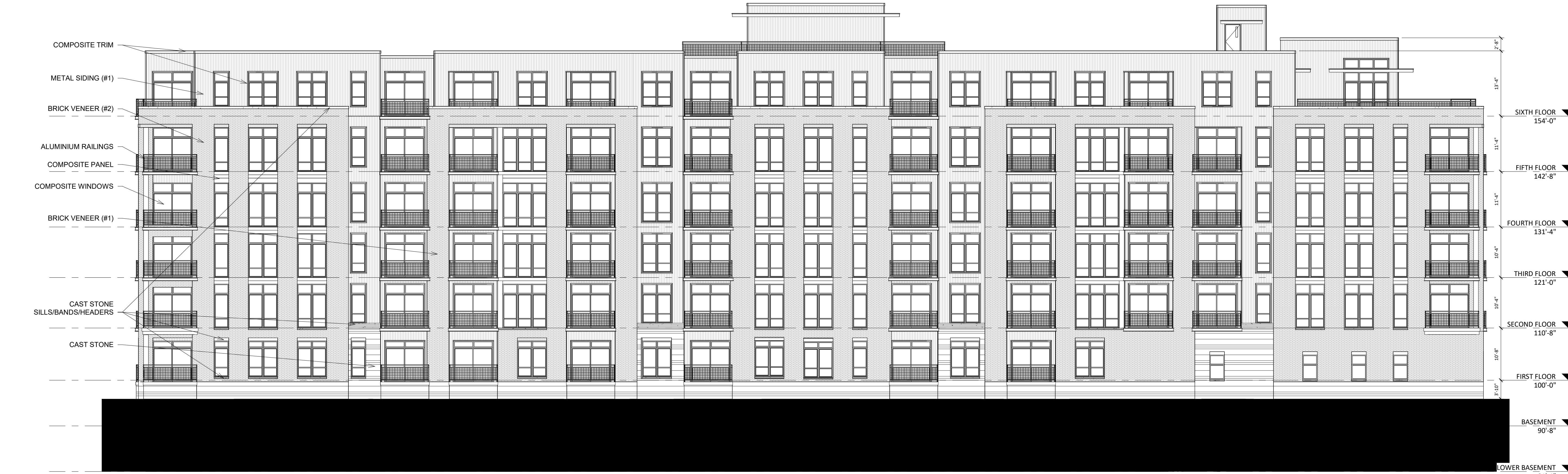
2 ELEVATION - SOUTH A-2.1 3/32" = 1'-0"
