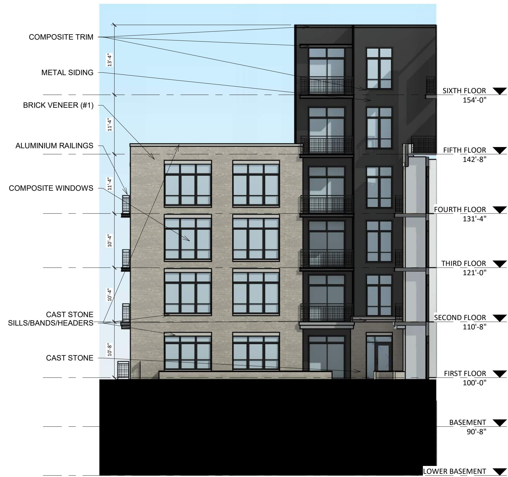
1 COLORED - ELEVATION - COURTYARD A-1 A-2.6 3/32" = 1'-0"
