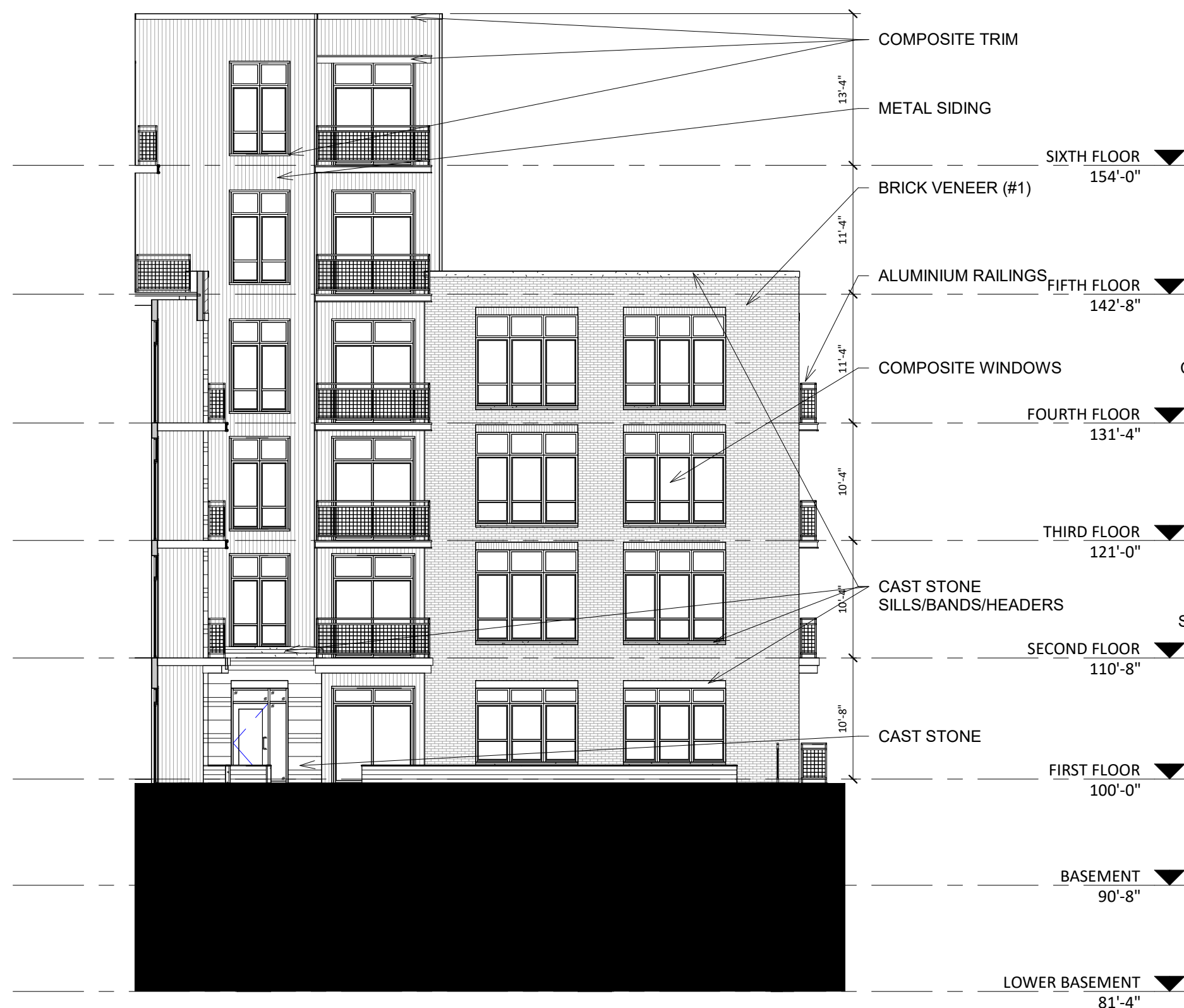
3 ELEVATION - COURTYARD B-1 A-2.3 3/32" = 1'-0"
