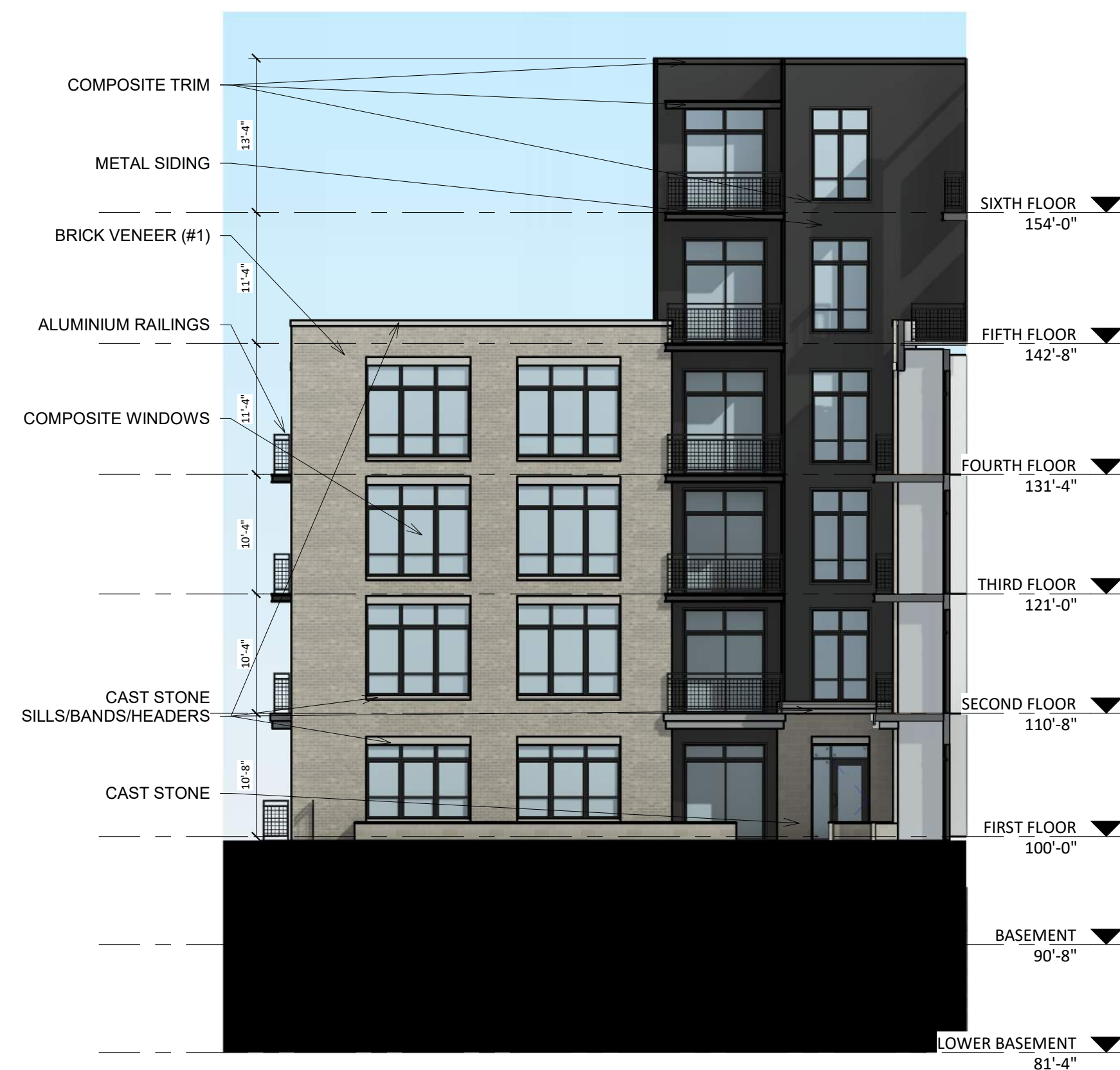
1 COLORED - ELEVATION - COURTYARD A-1 A-2.6 3/32" = 1'-0"
