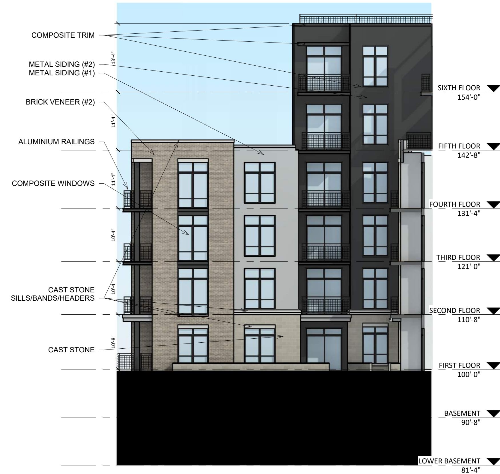
4 COLORED - ELEVATION - COURTYARD B-2 A-2.6 3/32" = 1'-0"
