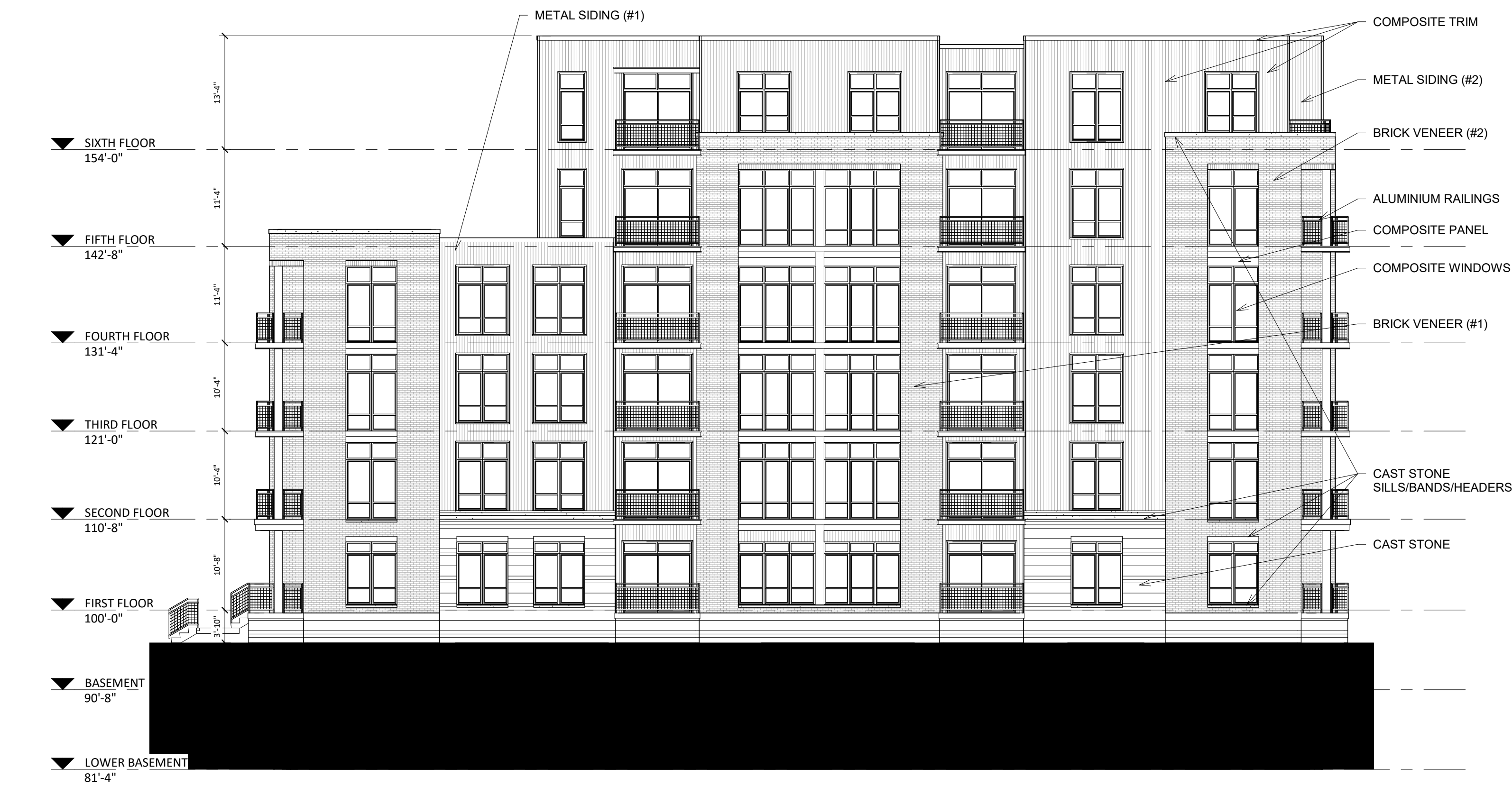
2 ELEVATION - WEST A-2.2 3/32" = 1'-0"
