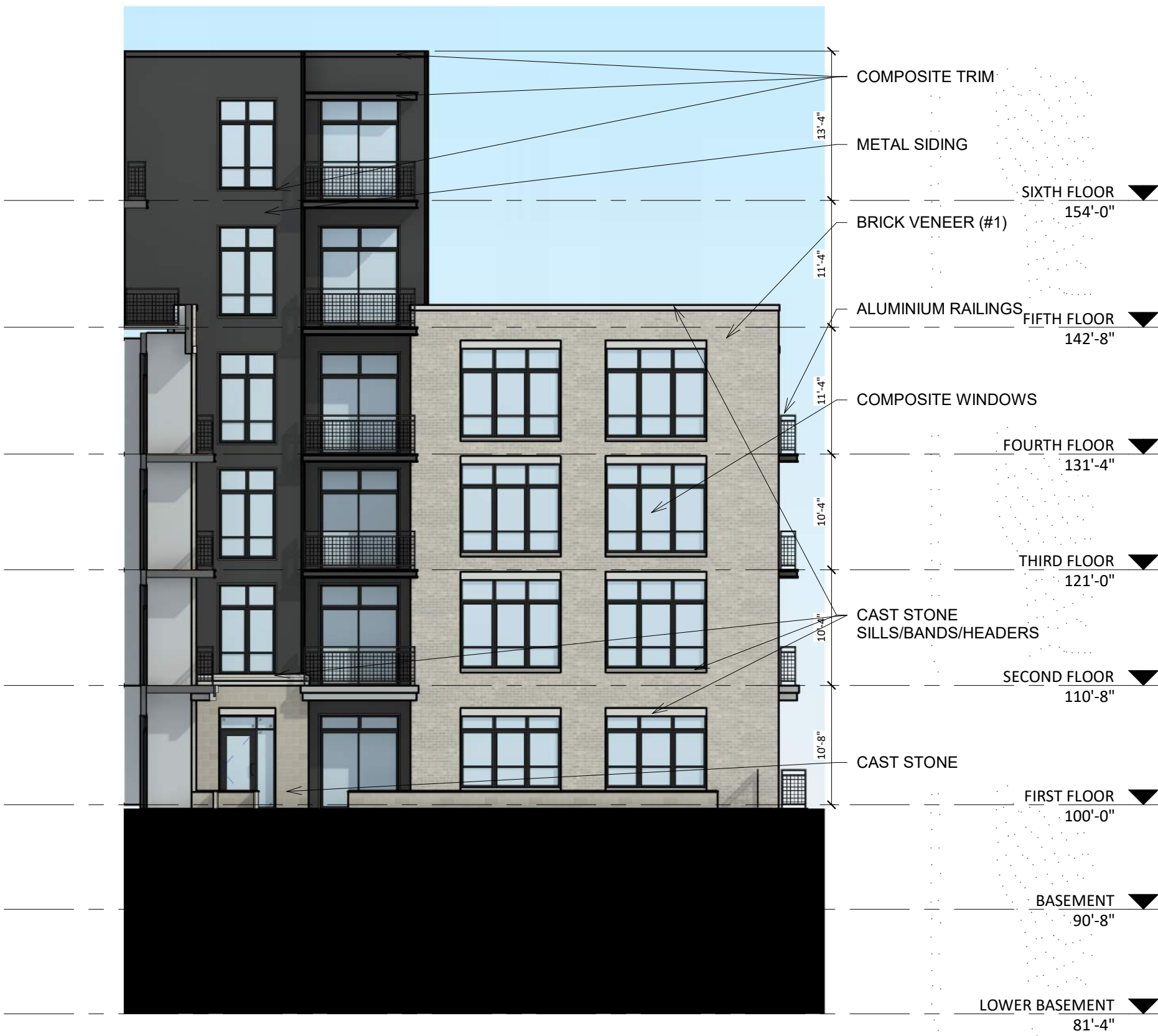
3 COLORED - ELEVATION - COURTYARD B-1 A-2.6 3/32" = 1'-0"
