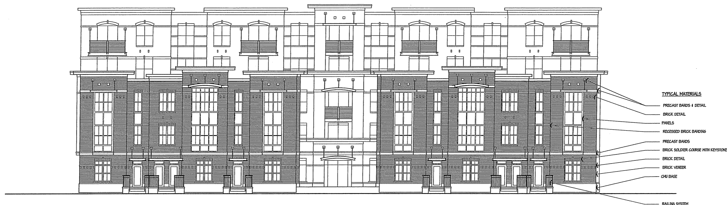
○ FRONT ELEVATION ALONG E. MIFFLIN STREET 1/8" = 1'-0"
