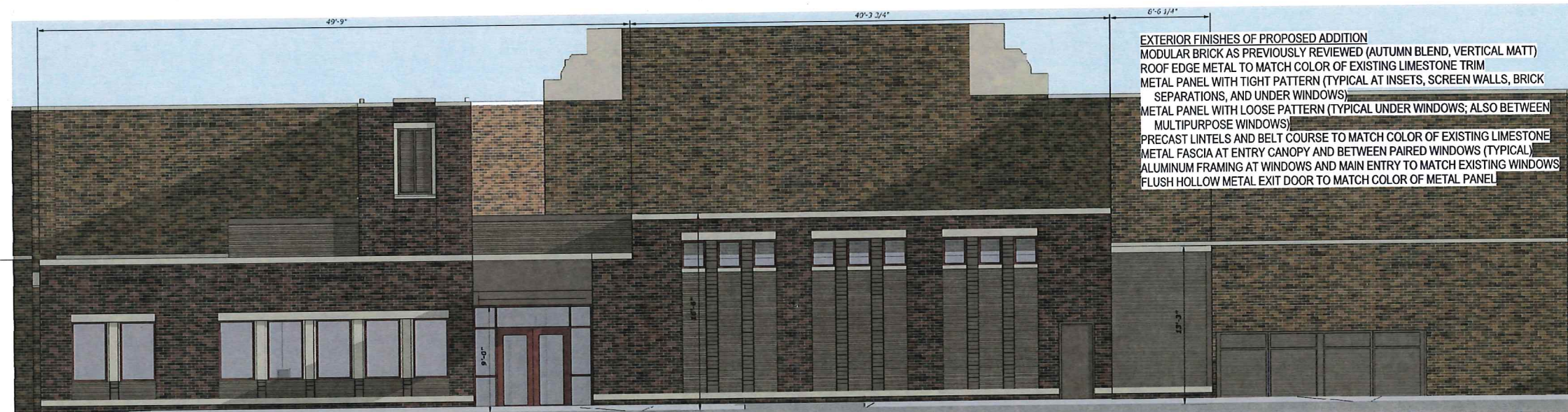
B1 PARTIAL PROPOSED NORTH ELEVATION 1/8" = 1'-0"
