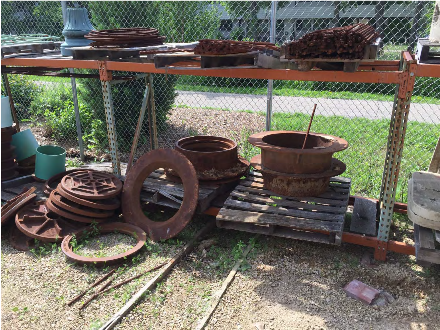
Traffic Engineering Yard M-9 : Manhole Lids and Rims
