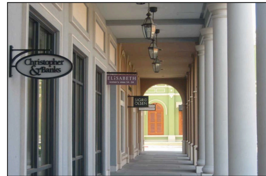
F SAMPLE RETAIL FLAG SIGNS 6 SQ FT MAX, 10 FT CLEAR TO GRADE.
