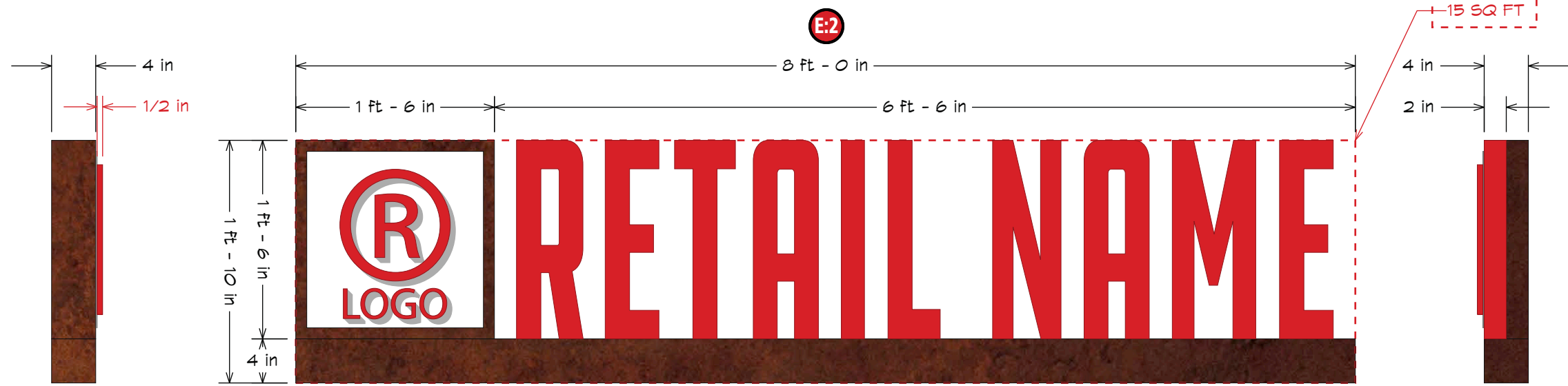
E:2 SAMPLE RETAIL SIGN - ABOVE CANOPY MOUNT INTERNALLY ILLUMINATED ALUMINUM LOGO LIGHT BOX WITH 4" RETURN & DETACHABLE FACE MOUNTED TO 4" ALUMINUM WIREWAY (FAUX CORTEN FINISH), ALUMINUM CHANNEL LETTERS OR ALUMINUM REVERSE CHANNEL LETTERS WITH SPLASH PLATE (COLORS SPECIFIC TO RETAIL CLIENT) MOUNTED TO TOP OF WIREWAY. 120V/20 AMP POWER ON DEDICATED BREAKER WITH PHOTOCELL & EXTERNAL POWER CUT-OFF SWITCH. POWER PULLED THROUGH CONDUIT TO WIREWAY. SIGN LOADS TO TOP OF CANOPY AT RETAIL ENTRANCE WITH "L" BRACKETS.
