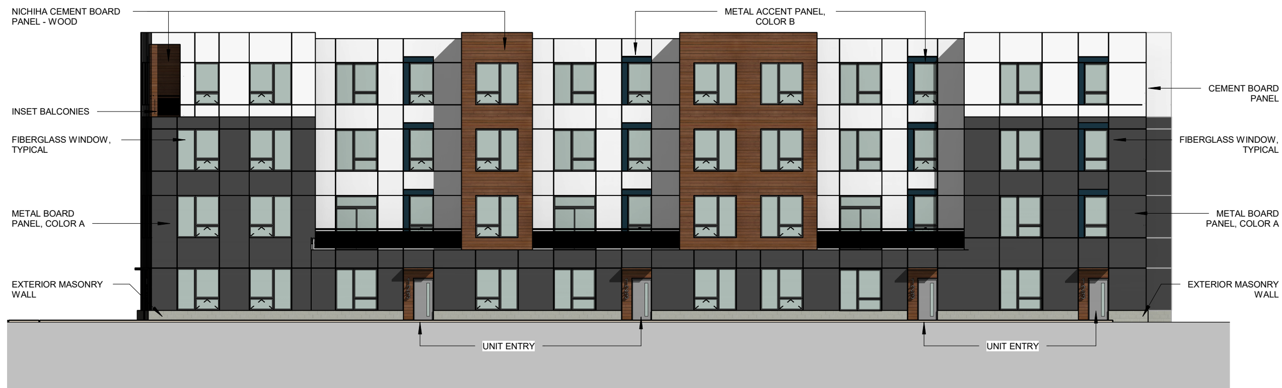
1 NORTH ELEVATION - OPTION 1 SCALE: 1/16" = 1'-0"
