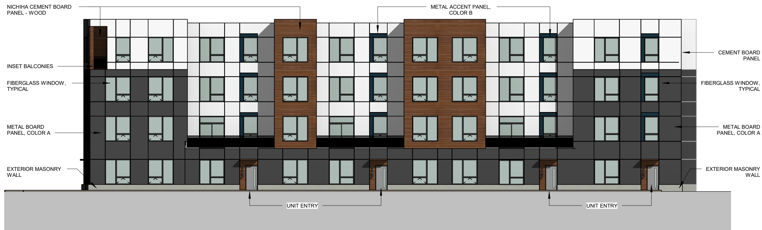
1 NORTH ELEVATION - OPTION 1 SCALE: 1/16" = 1'-0"
