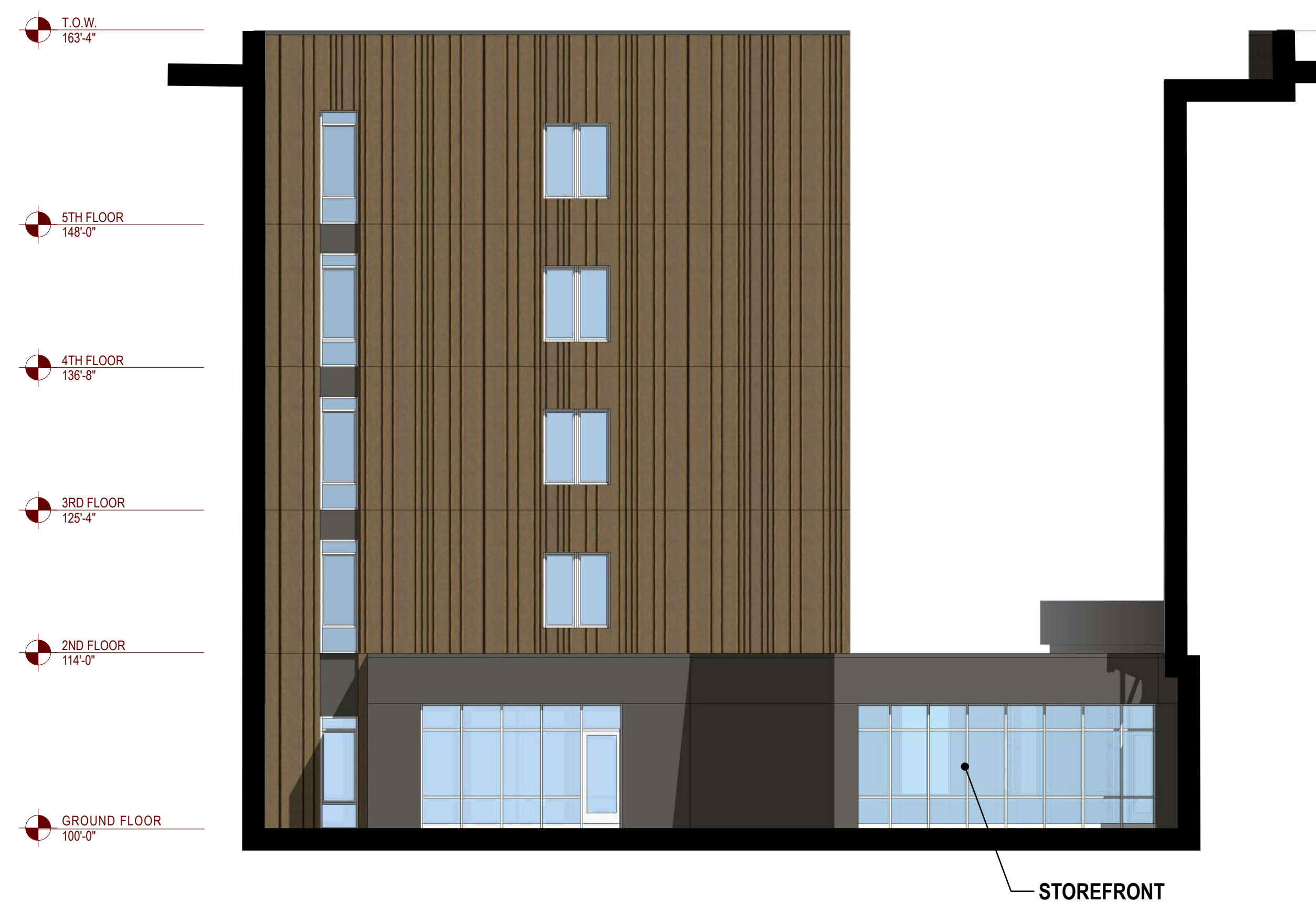
6 WEST BLDG. - SOUTH COURTYARD ELEVATION 1/8" = 1'-0"
