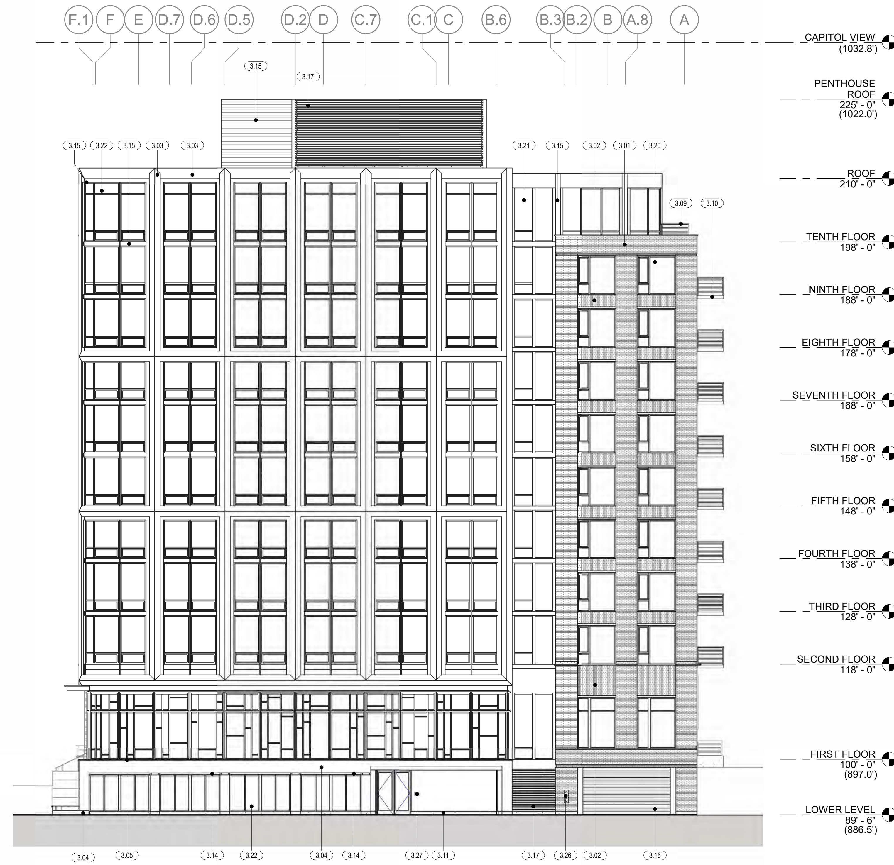
2 NORTHEAST ELEVATION - (NORTH HANCOCK STREET) A201 3/32" = 1'-0"
