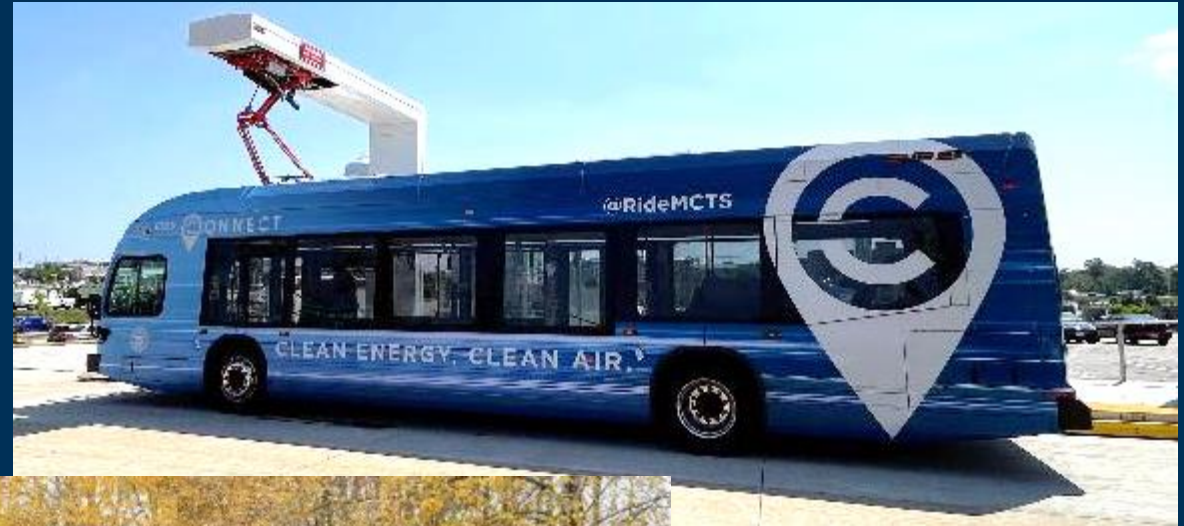
Photo: Over-head charging on Milwaukee's East-West BRT line
