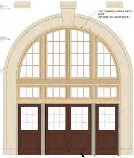
SOUTH ENTRY PAINT ELEVATION 1/8" = 1'-0"
