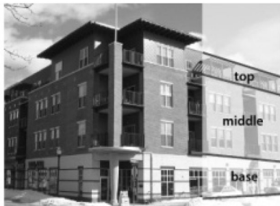
Figure D7: Building Articulation
