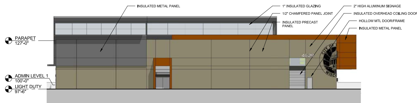
A8 PHASE 1A NORTHWEST ELEVATION 1/16" = 1'-0"
