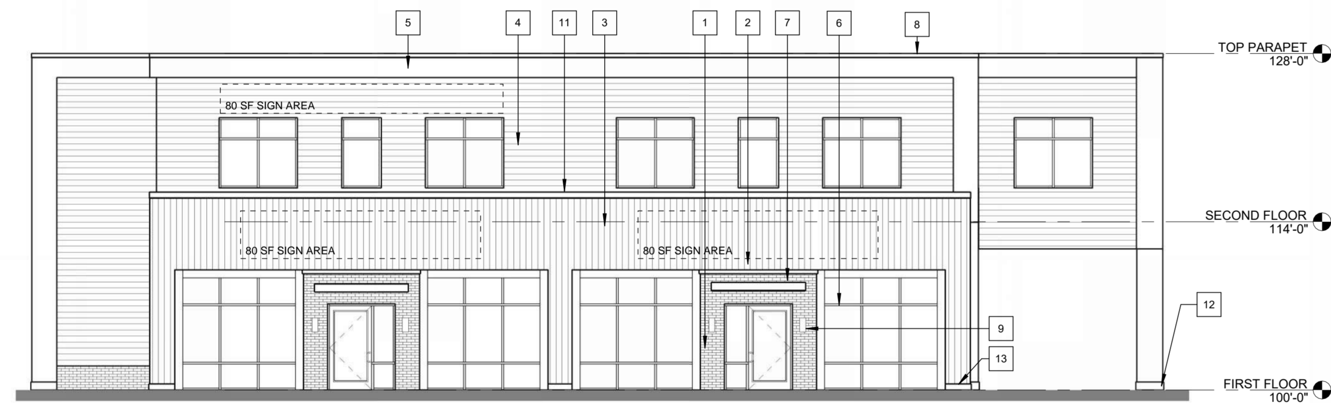
B1 NORTH ELEVATION (BW) 1/8" = 1'-0"
