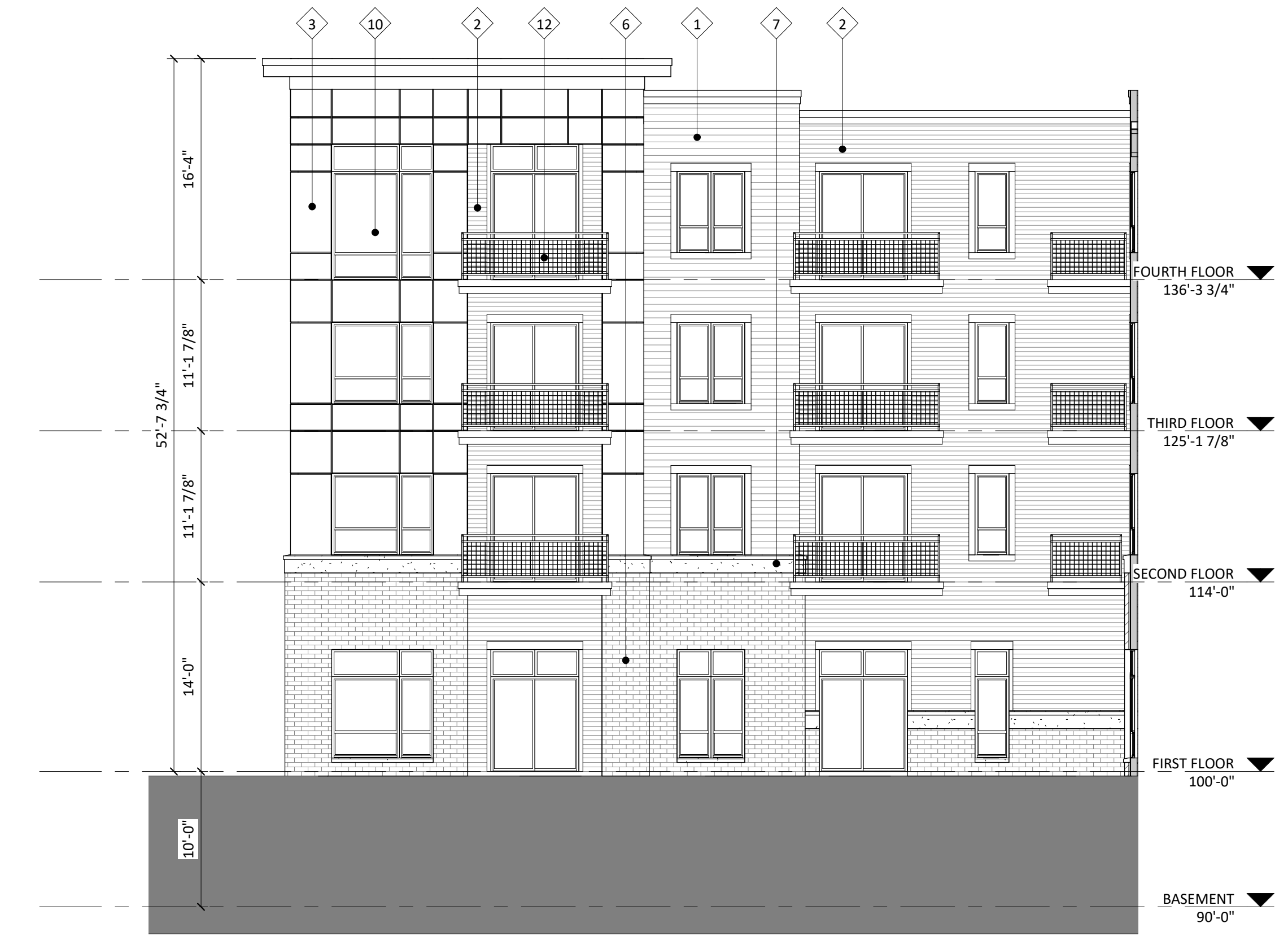
2 ELEVATION - EAST INTERIOR TERRACE A-2.2 1/8" = 1'-0"
