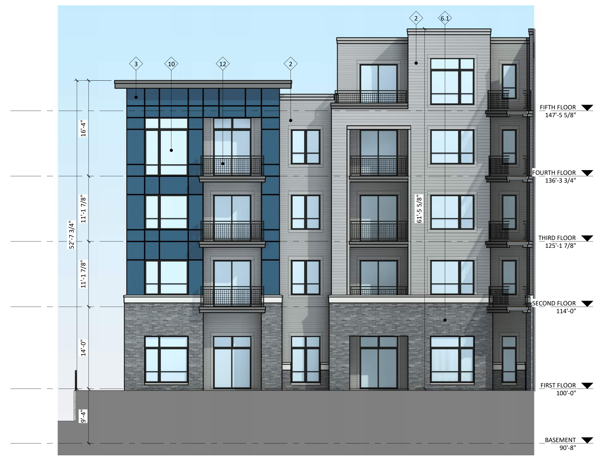
2 COLORED ELEVATION - NORTHWEST INTERIOR A-2.6 1/8" = 1'-0"
