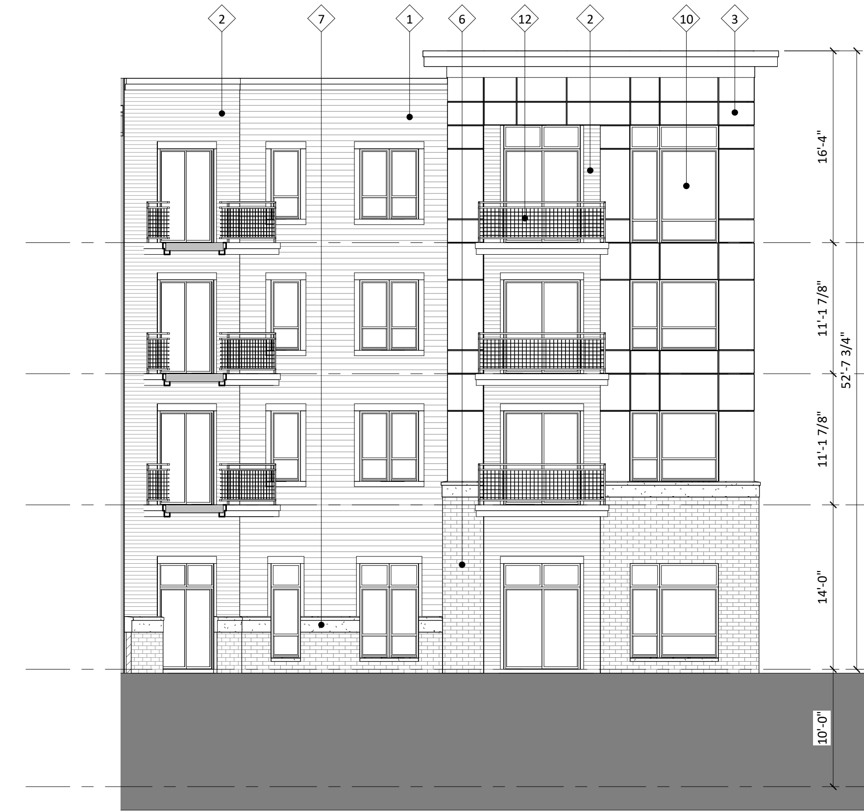
3 ELEVATION - WEST INTERIOR TERRACE A-2.2 1/8" = 1'-0"
