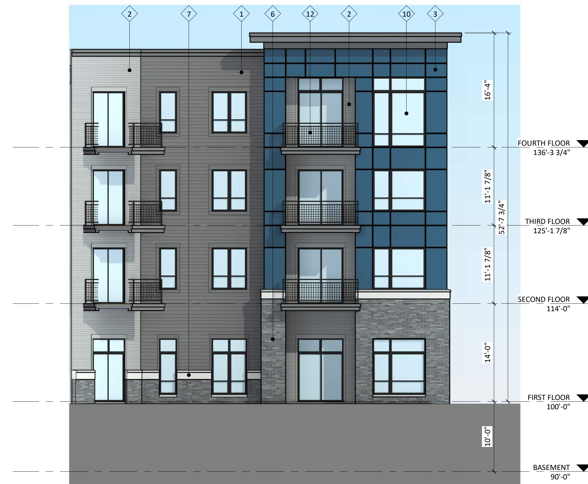
3 COLORED ELEVATION - WEST INTERIOR TERRACE A-2.5 1/8" = 1'-0"
