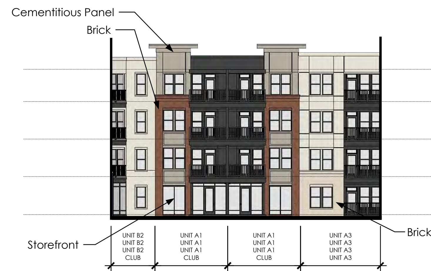
2 Pool Courtyard - East Elevation Scale: 1/16" = 1'-0" Elevation
