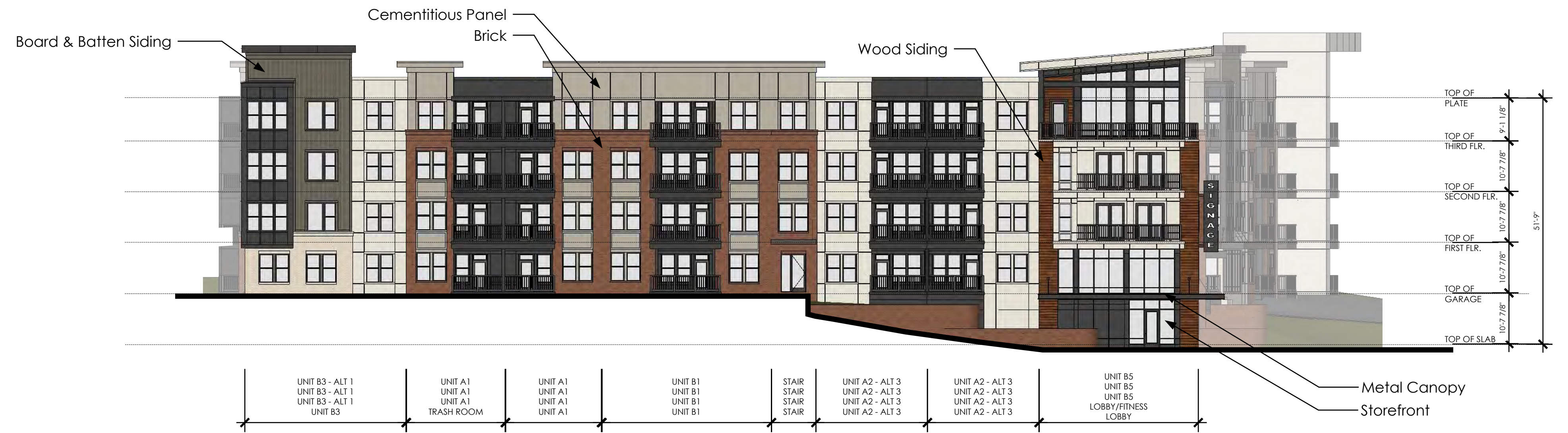
3 Left Elevation (West Elevation)
