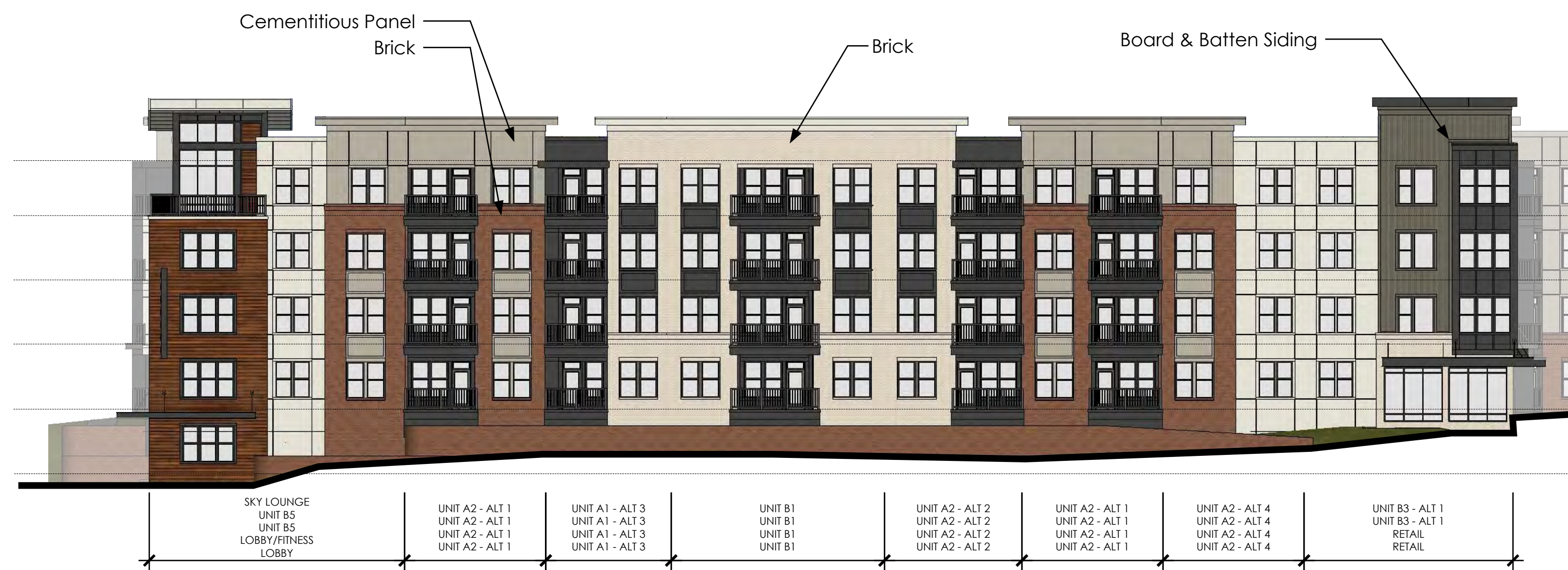
2 American Pkwy Elevation (South Elevation) Scale: 1/16" = 1'-0"
