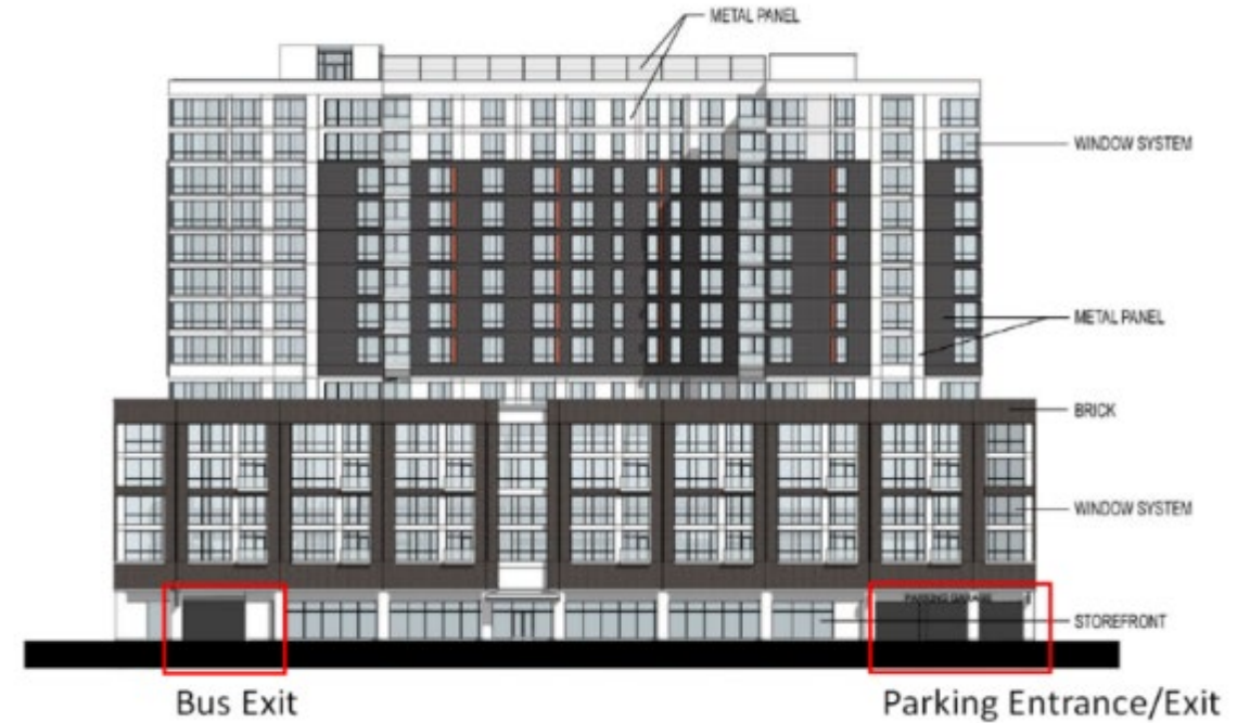
Figure 29 State Street Campus Mixed Use Development
