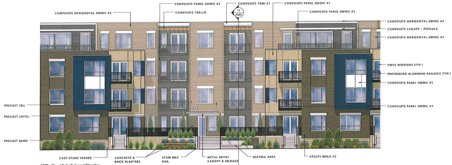
② Mifflin Street Entry Enlarged Elevation 1/8" = 1'-0"
