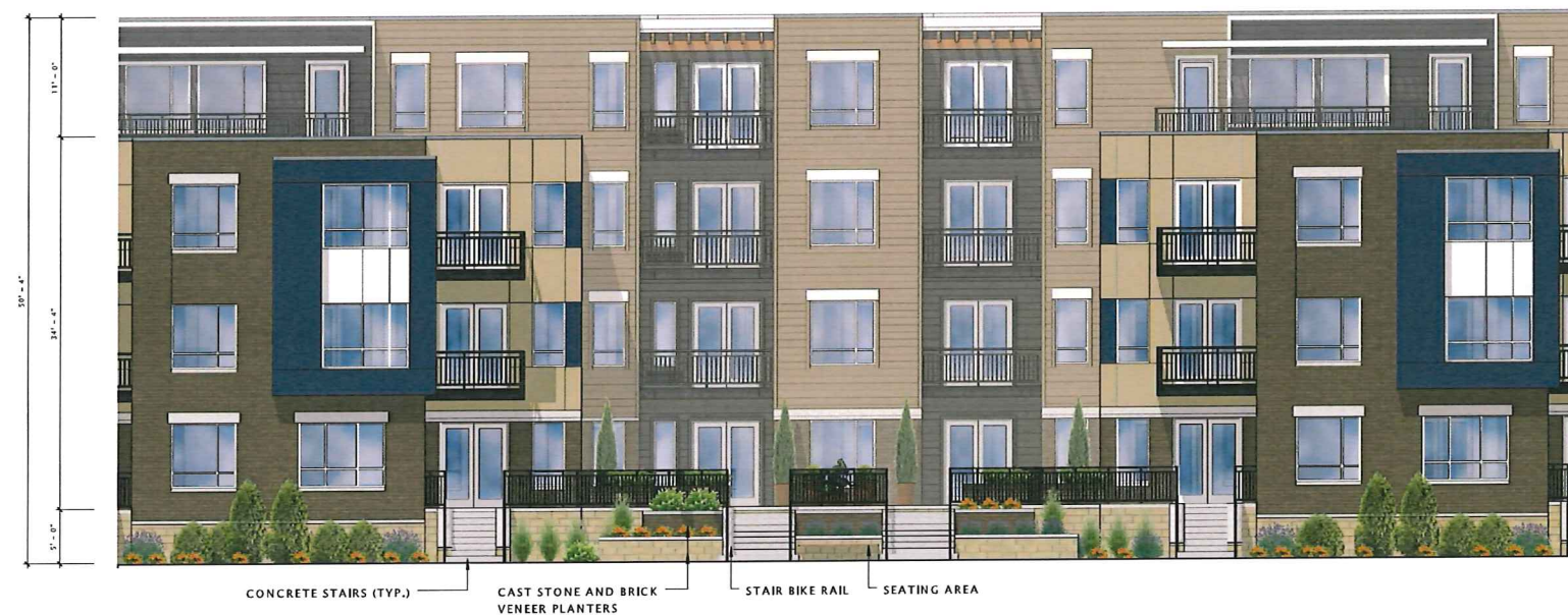
③ Mifflin Street Courtyard Enlarged Elevation 1/8" = 1'-0"
