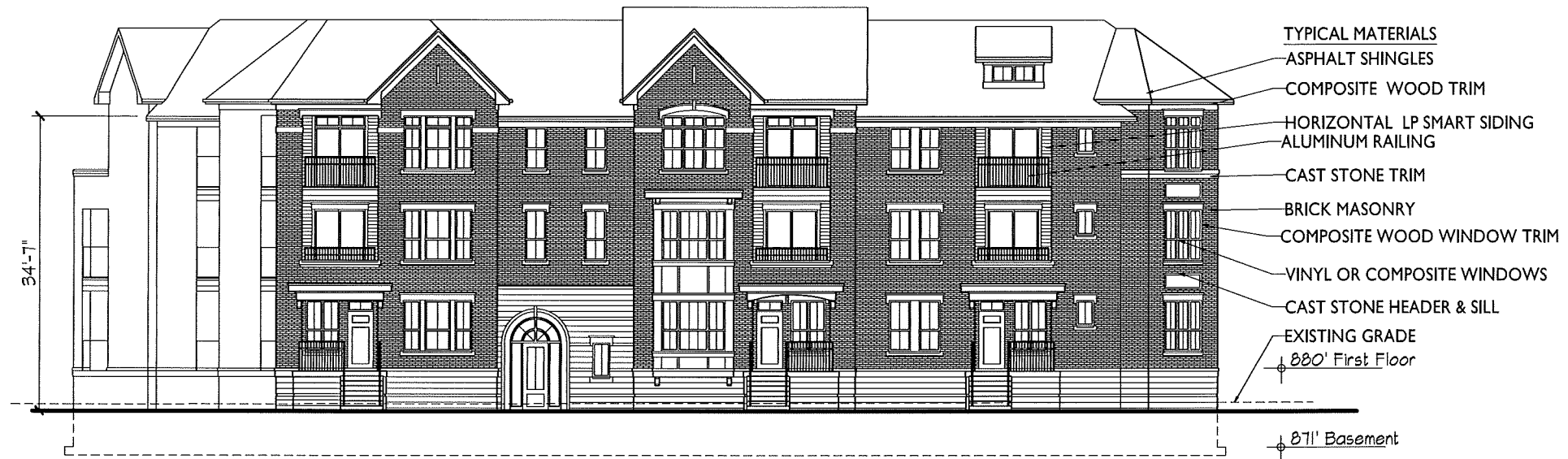
1 NORTH ELEVATION (ALONG UNIVERSITY AVE) A-2.1 1/8"=1'-0"
