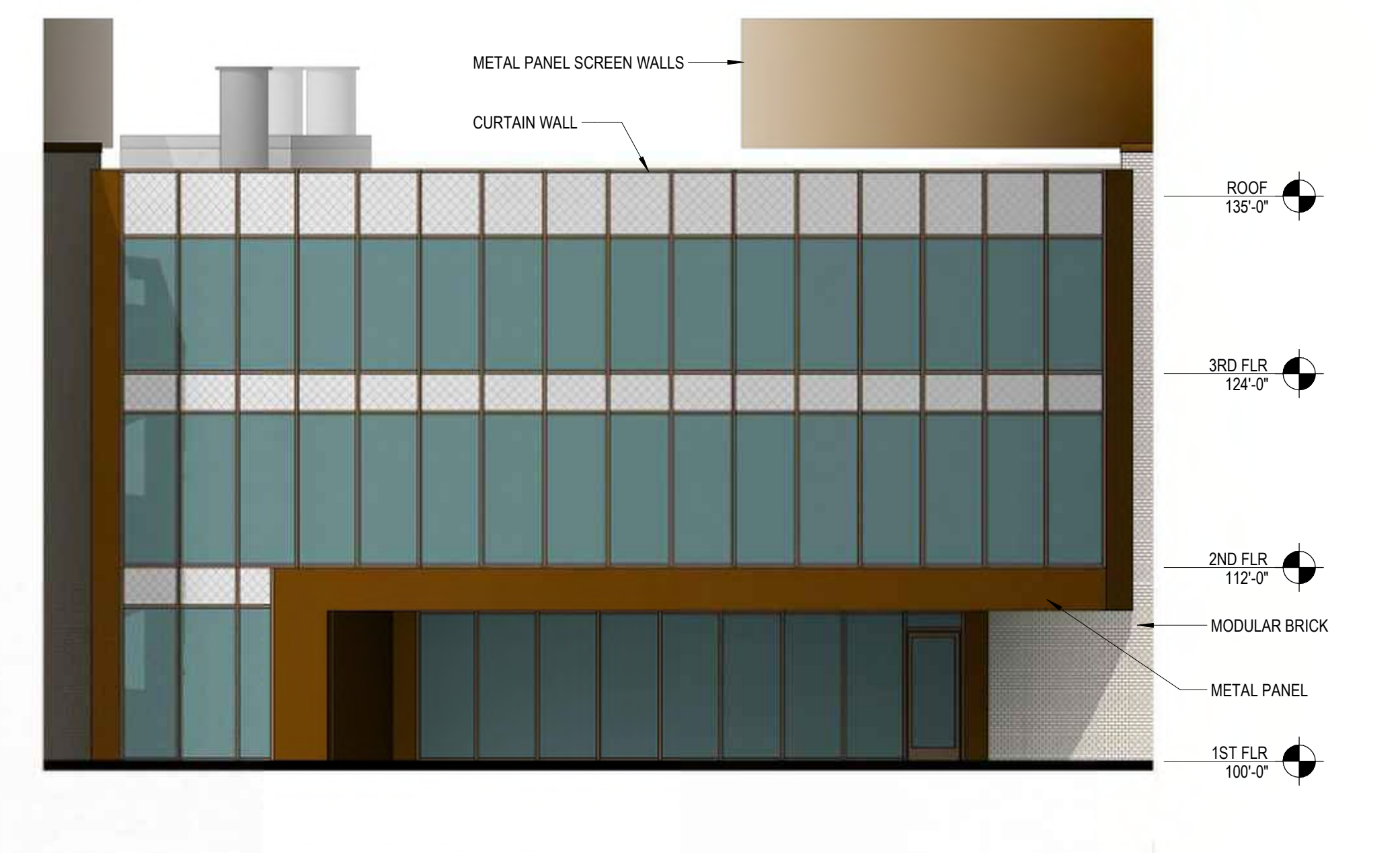
2 CENTRAL HUB - SW ELEVATION 1/8" = 1'-0"
