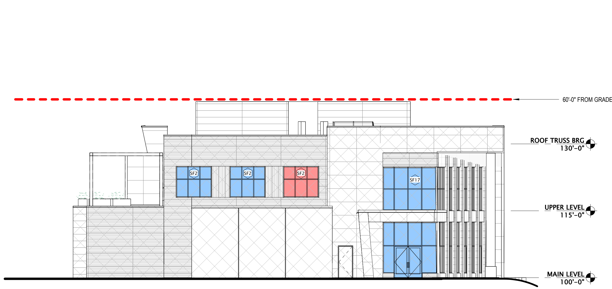
3 BIRD SAFE GLASS - EAST ELEVATION 3/32" = 1'-0"
