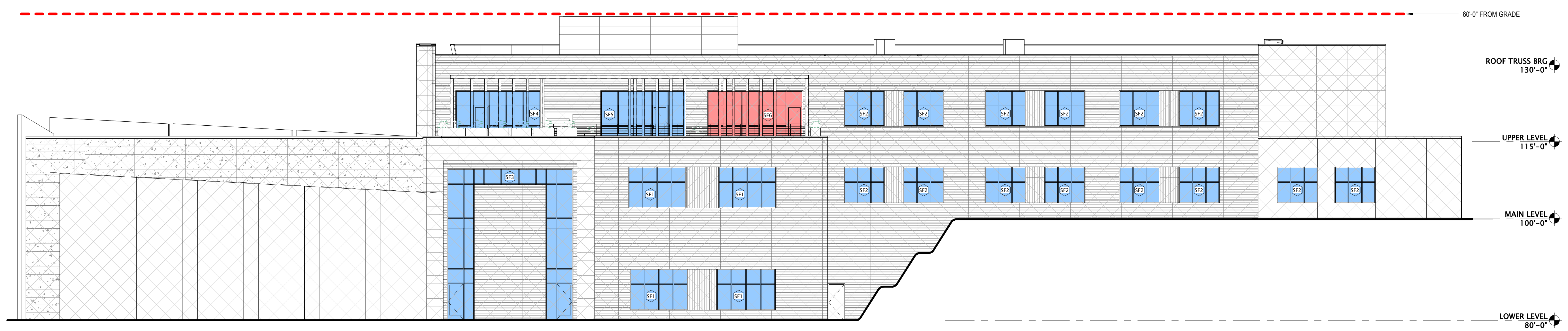
2 BIRD GLASS - SOUTH ELEVATION 3/32" = 1'-0"
