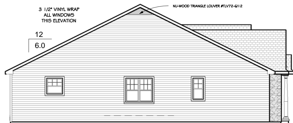
Left Elevation - Elevation C Stone 3/32" = 1'-0"
