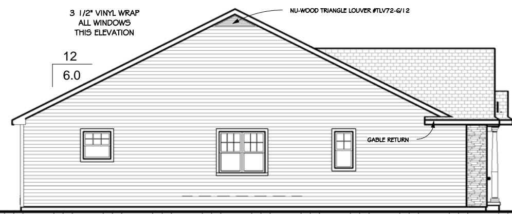
Left Elevation - Elevation C Stone 3/32" = 1'-0"
