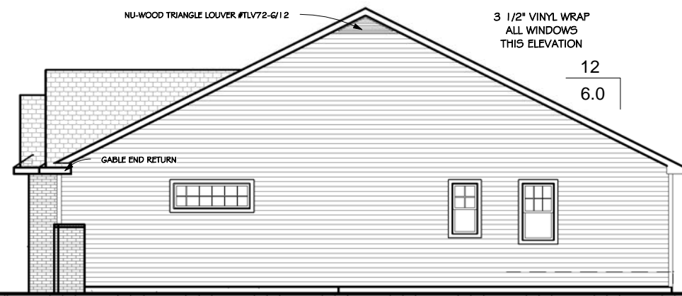
Right Elevation - Elevation B Brick 3/32" = 1'-0"
