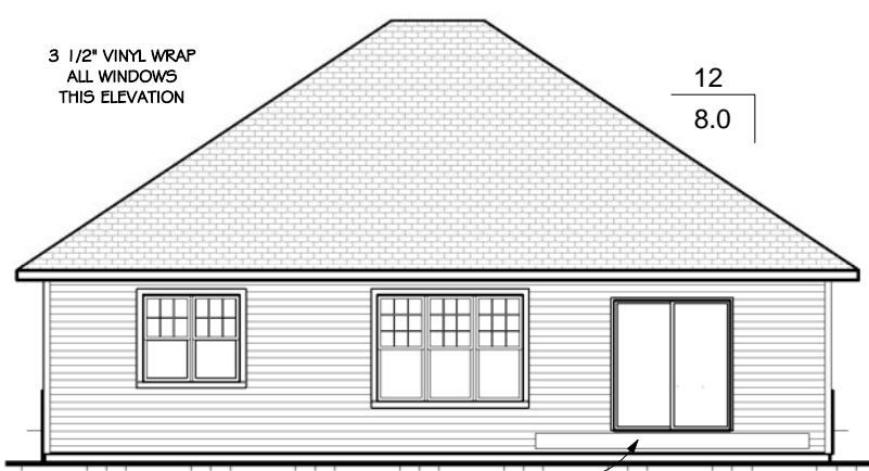
Rear Elevation - Elevation A Stone 3/32" = 1'-0"
