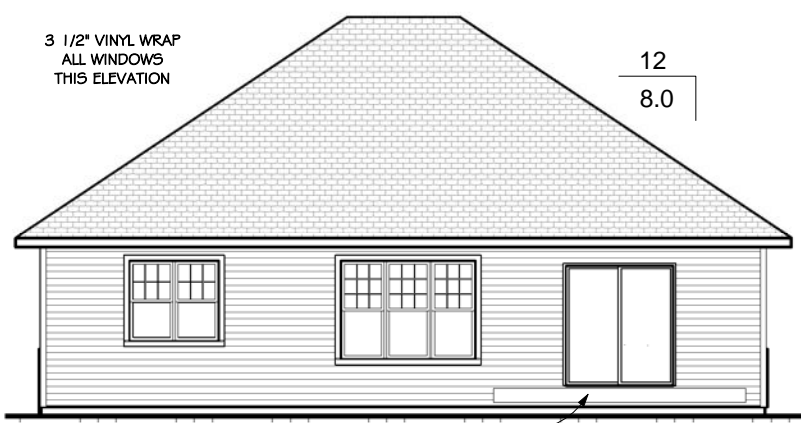
Rear Elevation - Elevation A Stone 3/32" = 1'-0"
