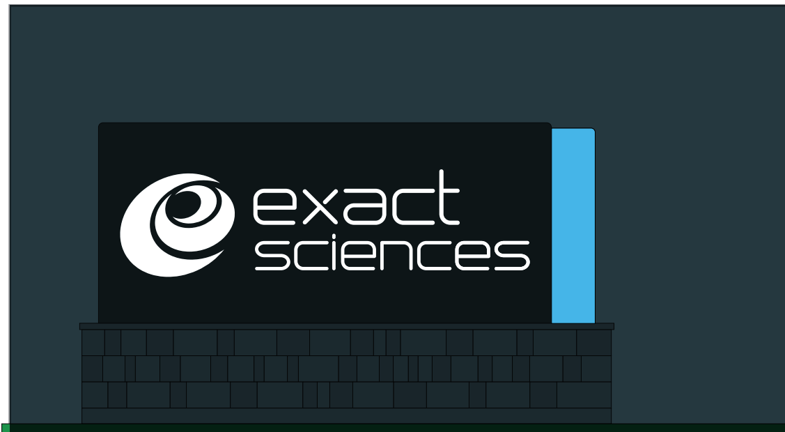
SIGN TYPE A - LARGE MONUMENT (DOUBLE-SIDED) NEW SIGN TO USE EXISTING MONUMENT STRUCTURE (INTERNALLY LIT)
