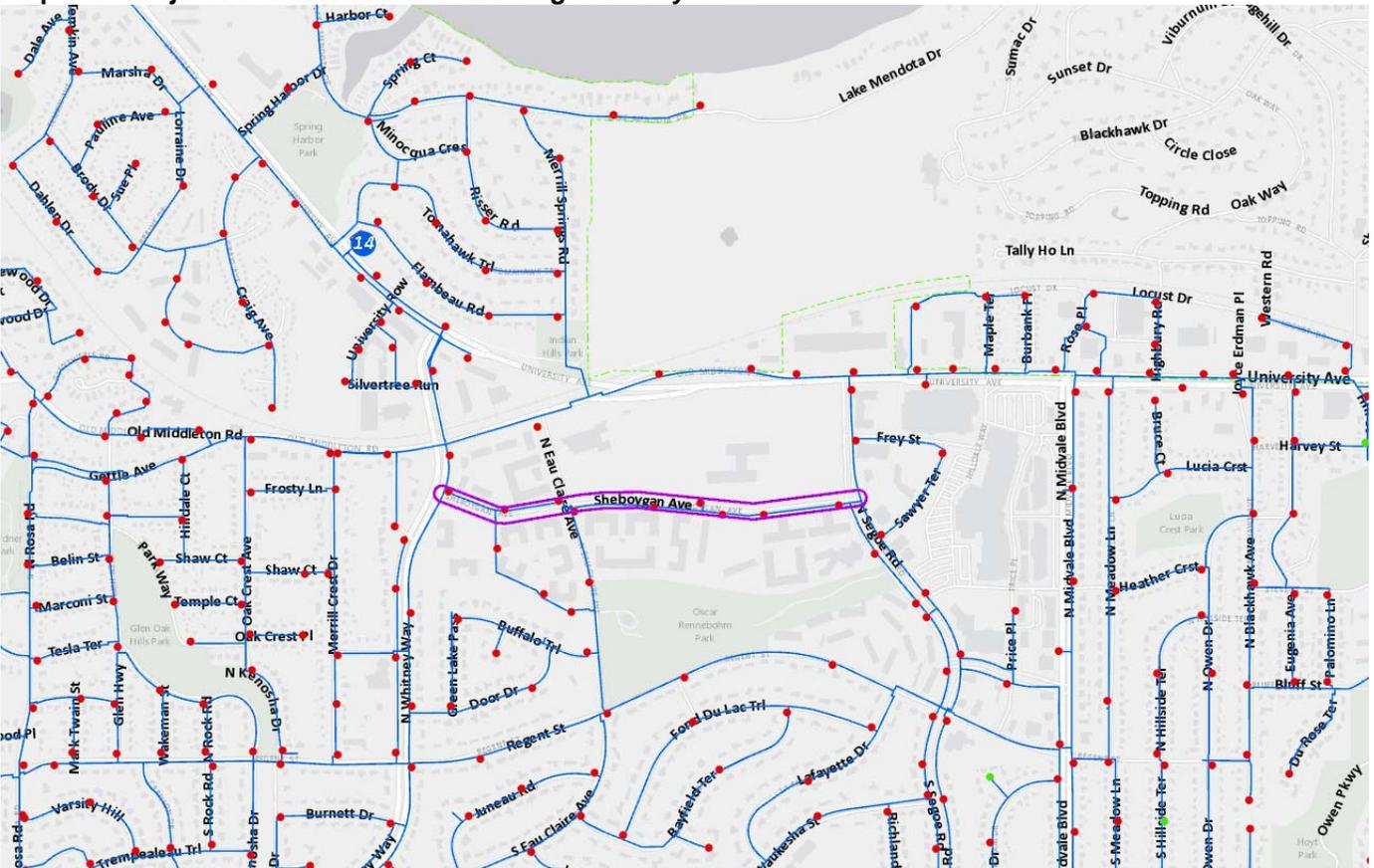
**Project Scope:** Proposed replacement of approximately 3,000-FT of existing mid-century 6-IN cast iron water mains with new 12-inch ductile iron water mains to improve fire flow capacity and water system hydraulics serving the Hill Farms DOT redevelopment site.
