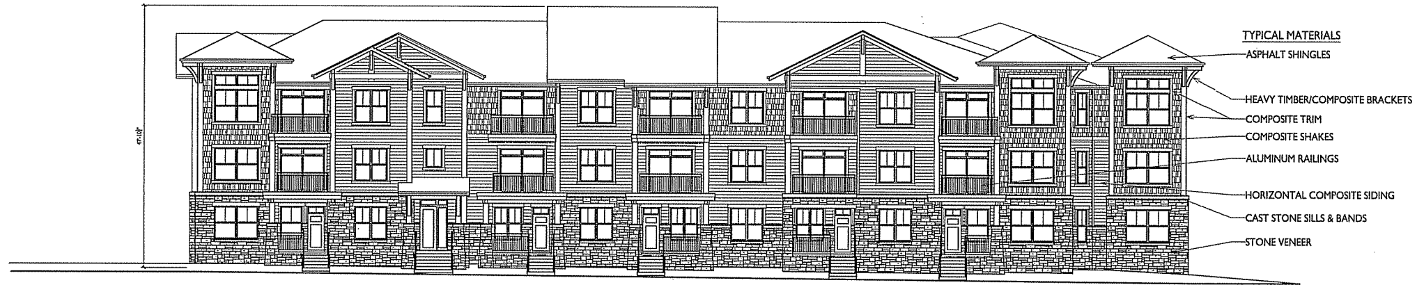
BUILDING 5 NORTHWEST ELEVATION 3/32"=1'-0"
