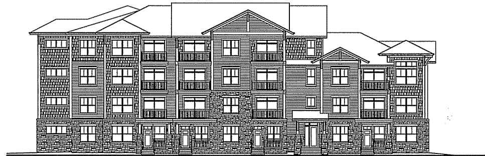
BUILDING 3 SOUTHWEST ELEVATION 1/16"=1'-0"
