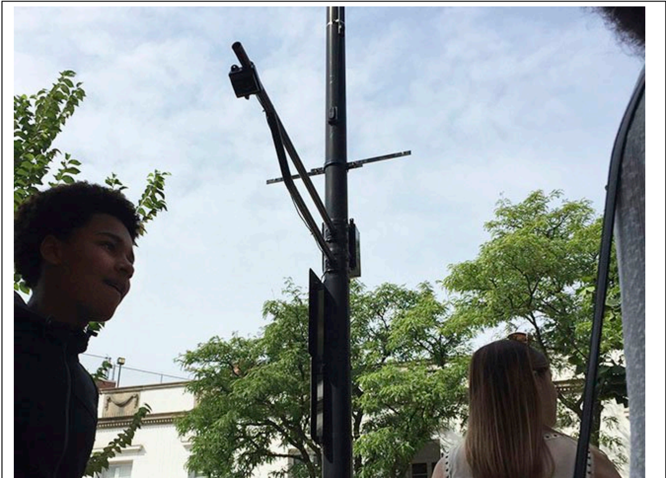
A passive infrared camera hanging over the 100 block of State Street counts pedestrians by detecting their body heat.
