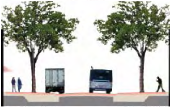
PEDESTRIAN ZONE 12'-0" FLEX ZONE 9'-0" CARWAY 24'-0" FLEX ZONE 9'-0" PEDESTRIAN ZONE 12'-0" SIDEWALK 21'-0" SIDEWALK 21'-0" Service "Flex"
