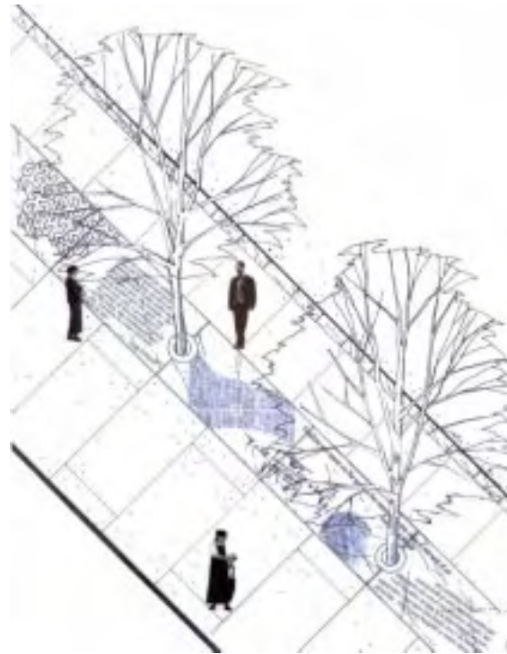
Granite paving - Alternate 2 Four-foot wide strip
