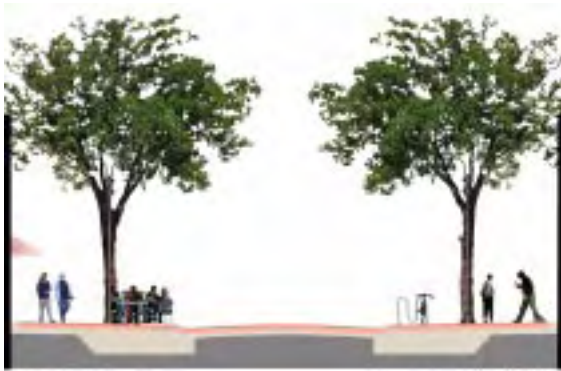
PEDESTRIAN ZONE 12'-0" FLEX ZONE 9'-0" CARWAY 34'-0" FLEX ZONE 9'-0" PEDESTRIAN ZONE 12'-0" SIDEWALK 21'-0" SIDEWALK 21'-0" Dining "Flex"
