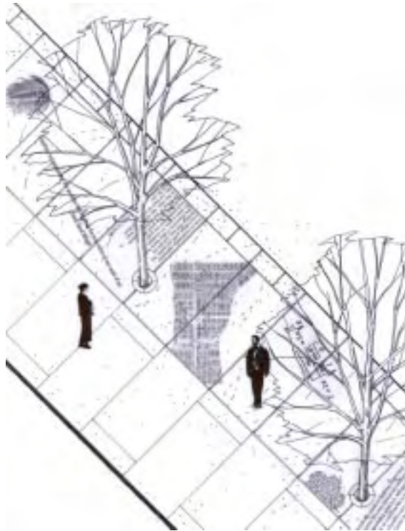
Granite paving - Alternate 1 Seven-foot wide strip
