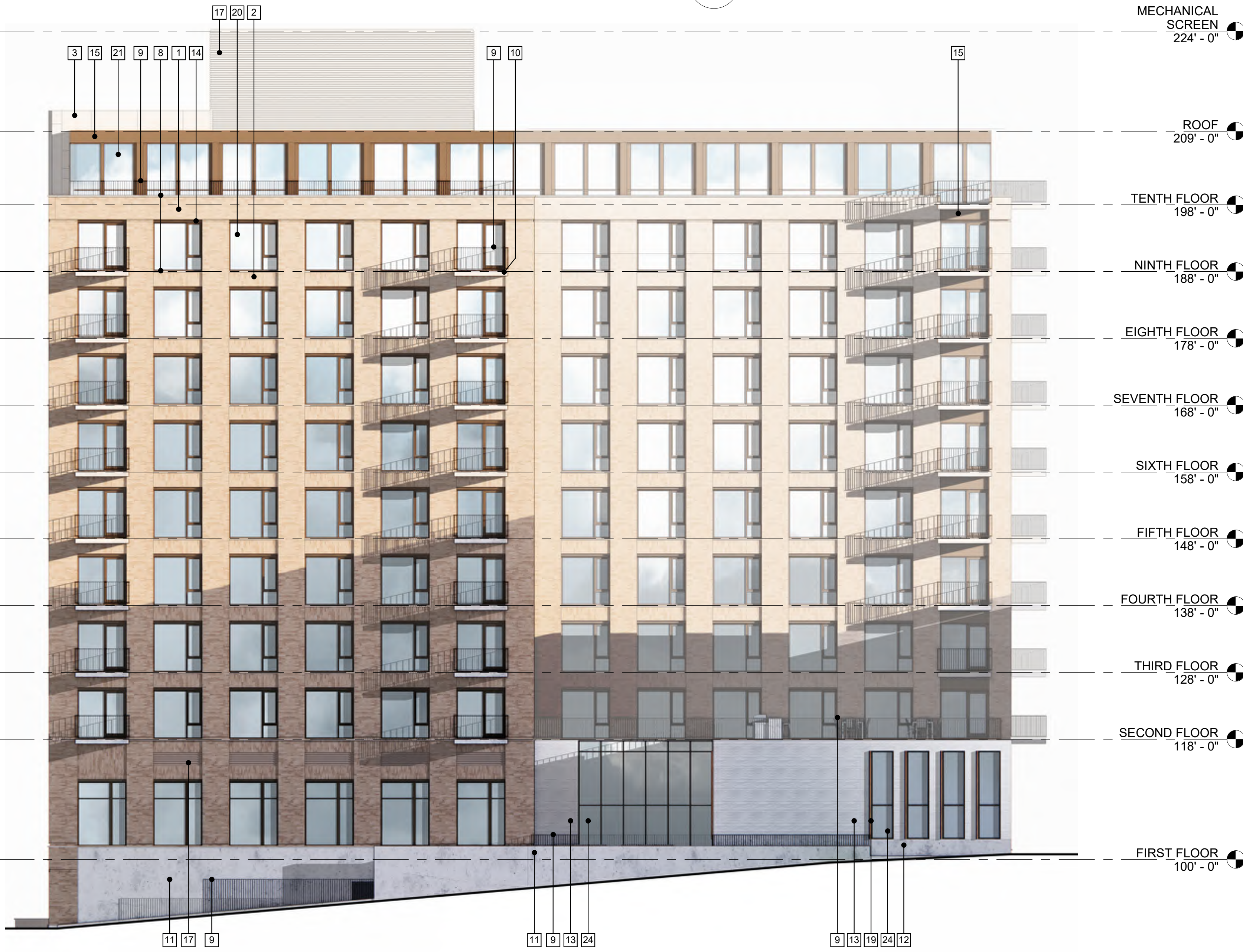
4 NORTH-WEST ELEVATION A250 3/32" = 1'-0"
