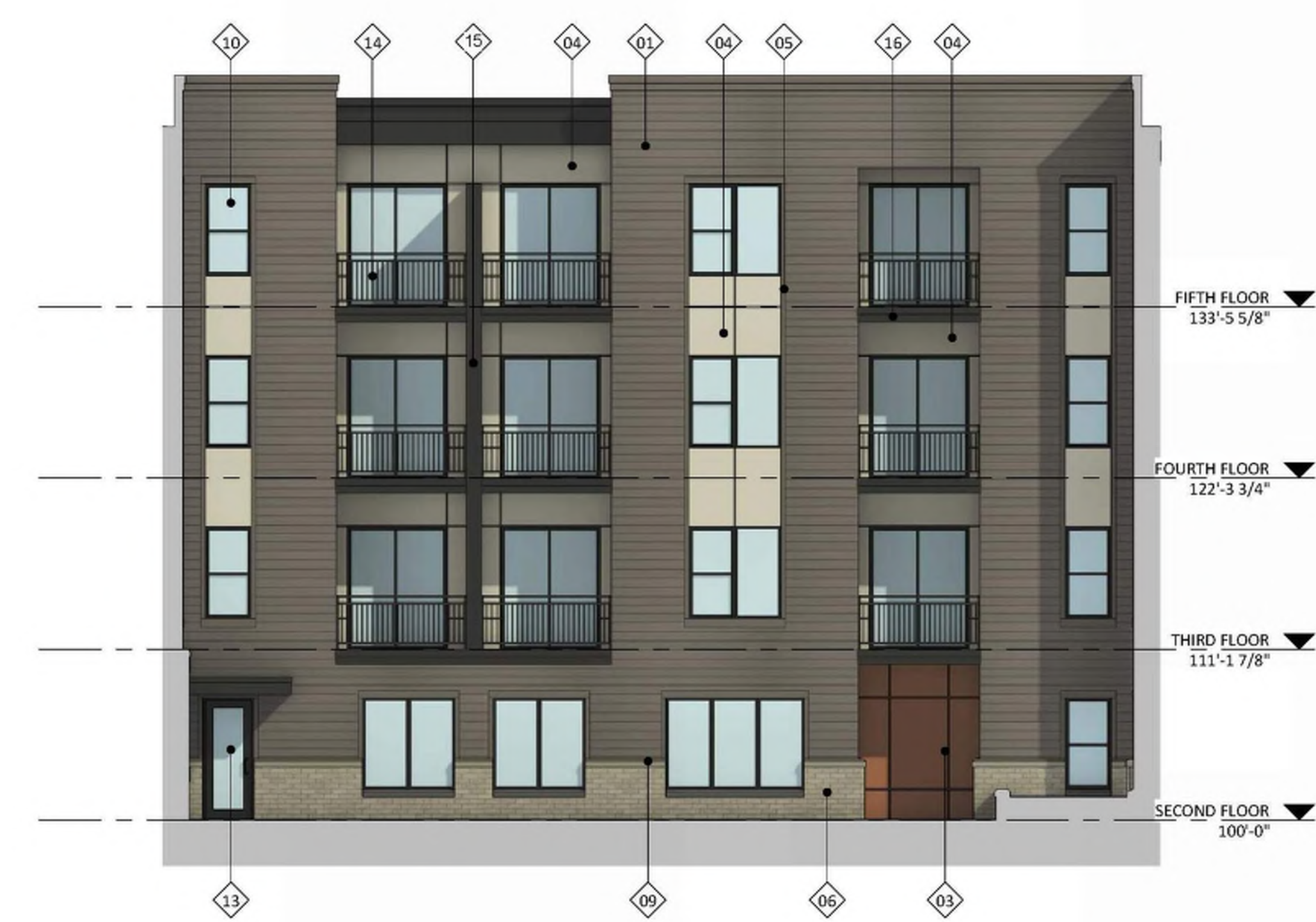
WEST COURTYARD ELEVATION
