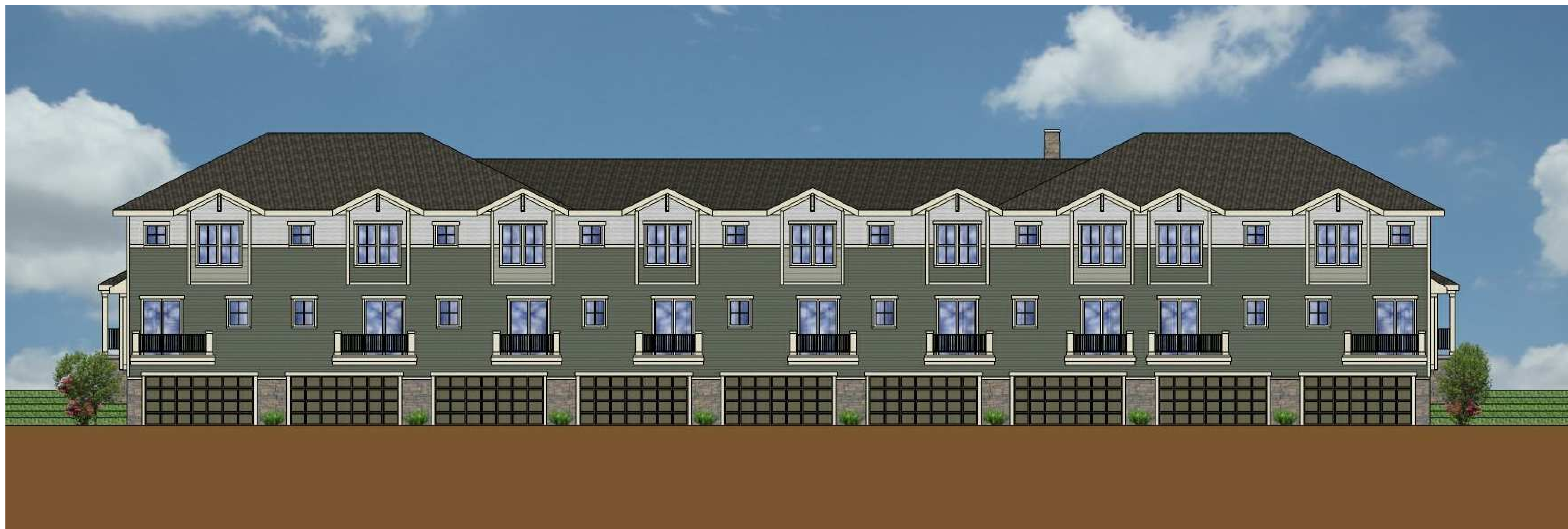
16 BUILDING 'F' - BACK ELEVATION 1/8" = 1'-0"
