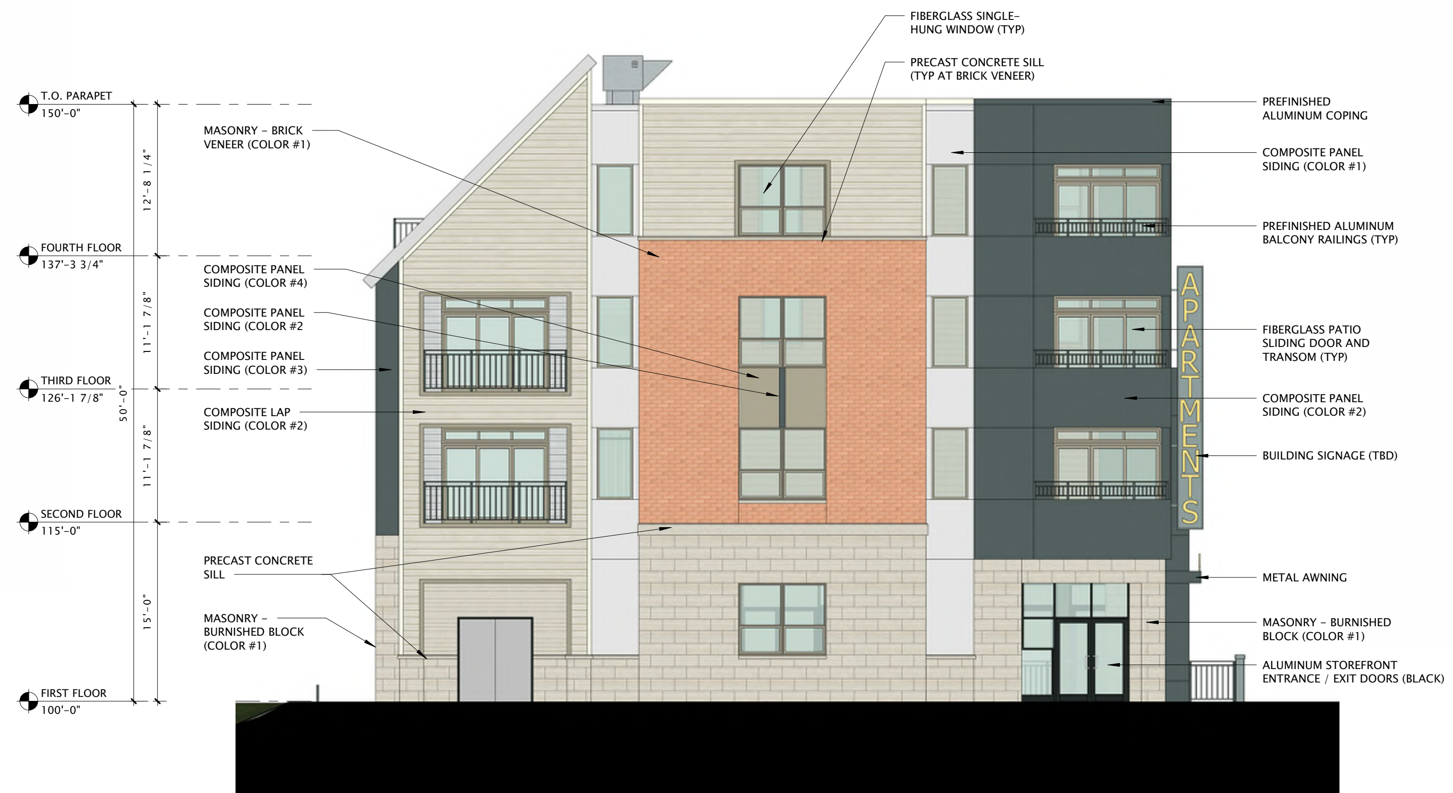
9 BUILDING 'A' - SOUTH ELEVATION 1/8" = 1'-0"
