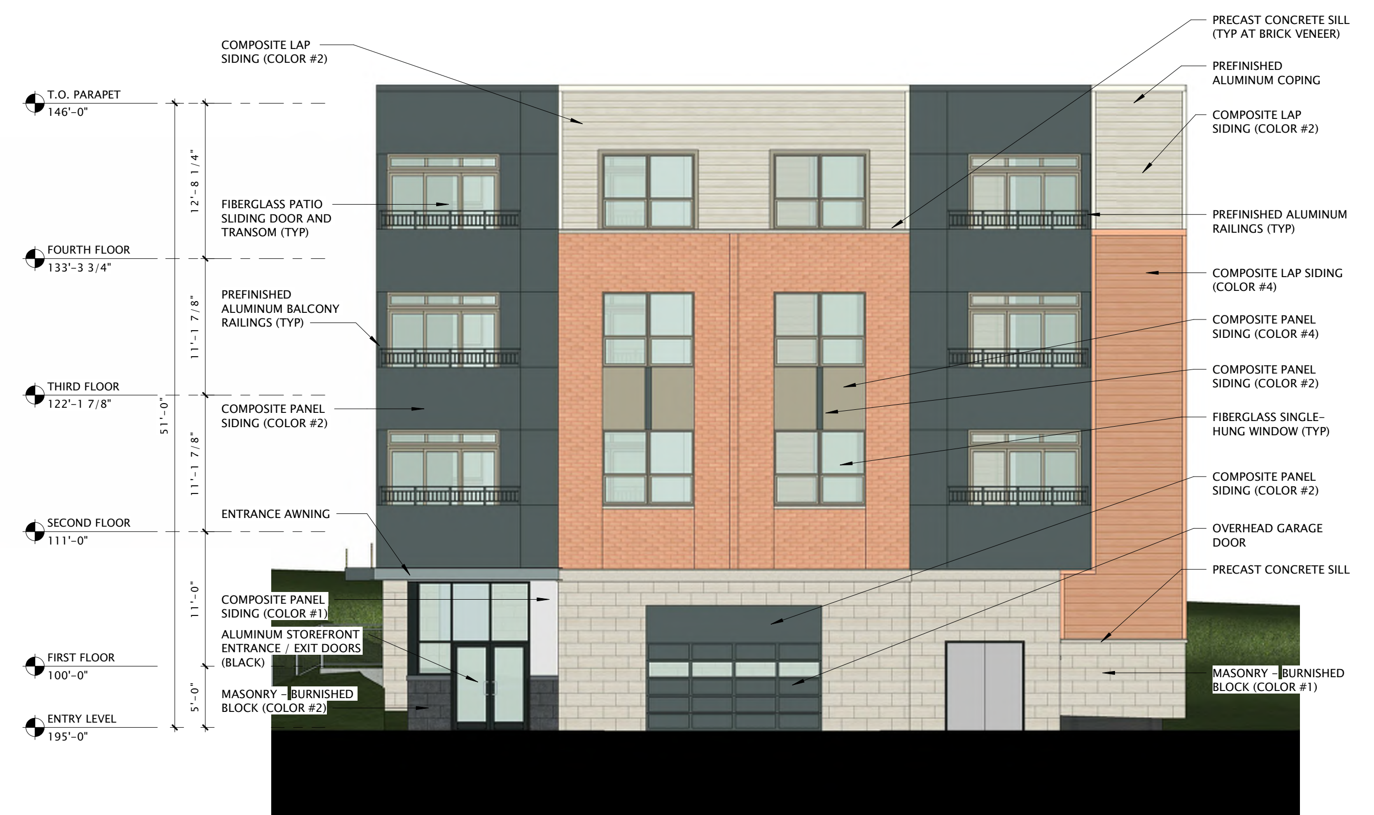
10 BUILDING 'C' - WEST ELEVATION 1/8" = 1'-0"
