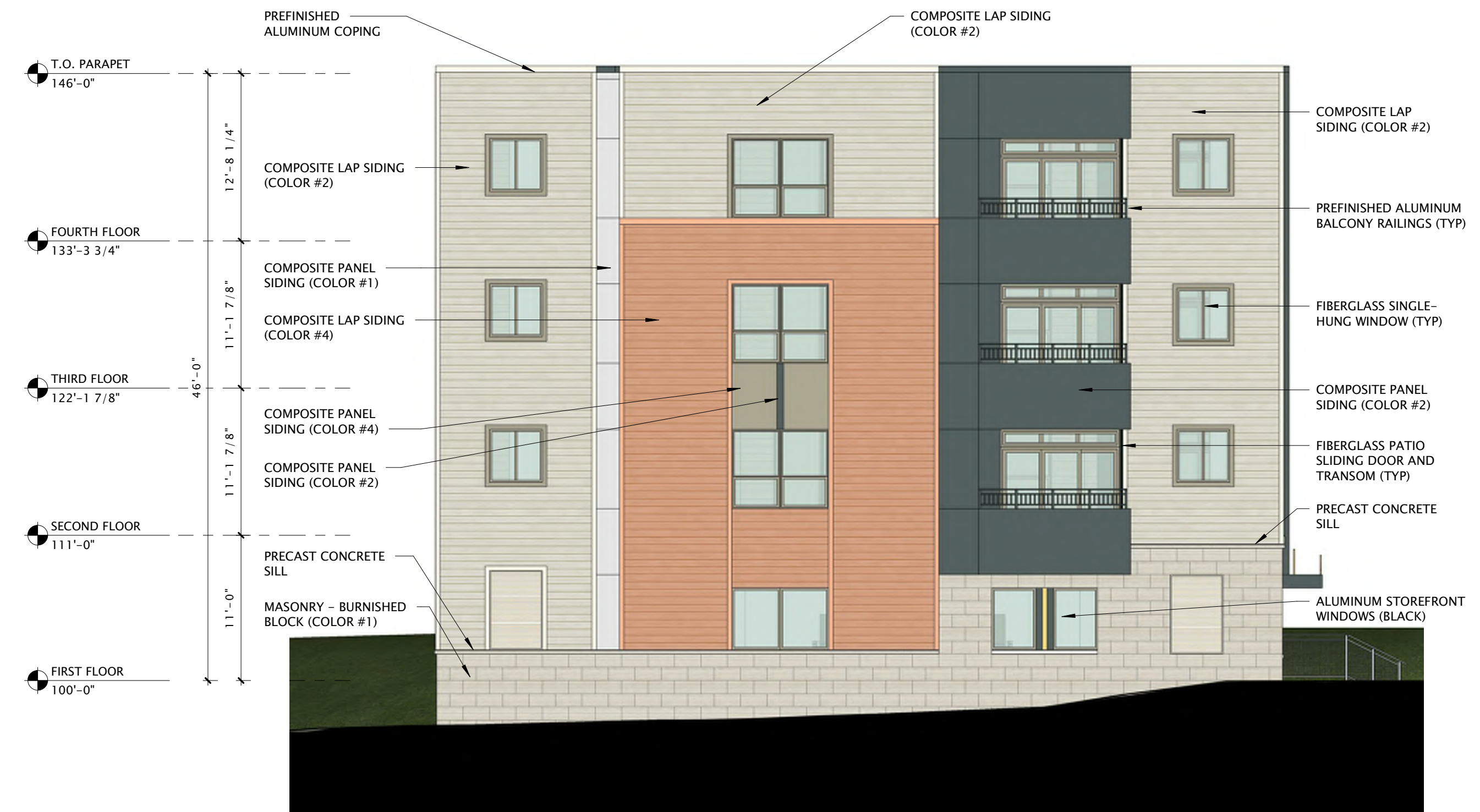
9 BUILDING 'C' - EAST ELEVATION 1/8" = 1'-0"
