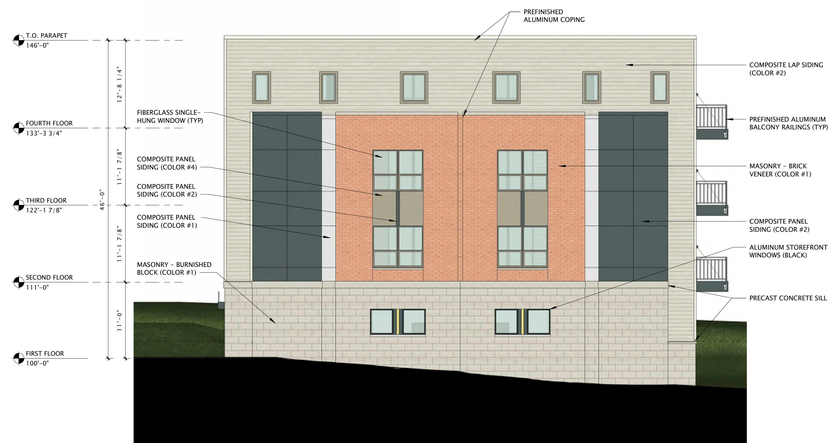
18 BUILDING 'B' - WEST ELEVATION 1/8" = 1'-0"
