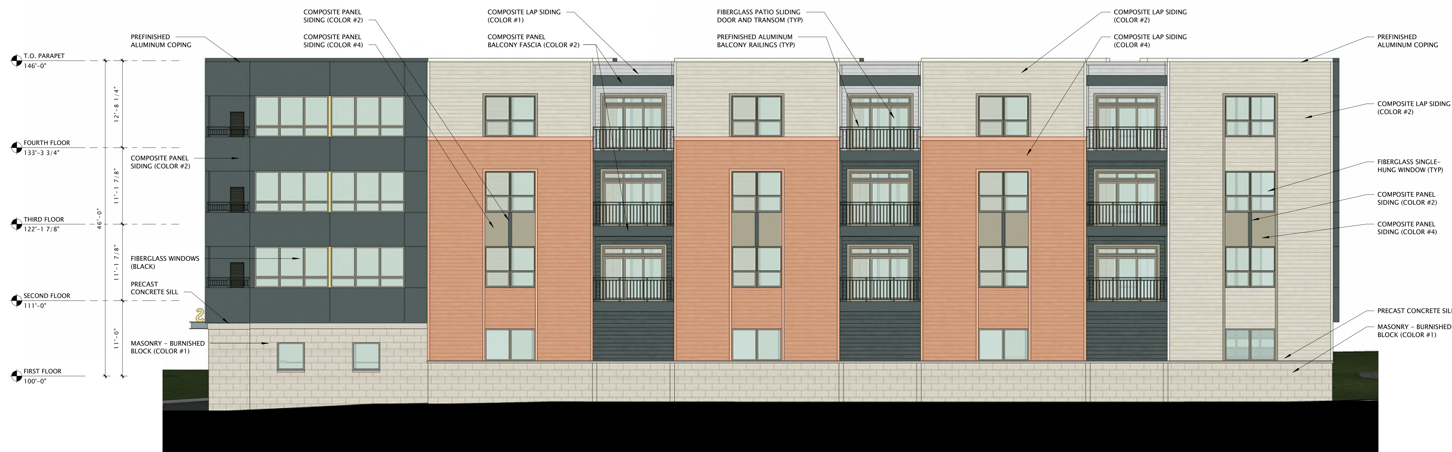
16 BUILDING 'C' - SOUTH ELEVATION 1/8" = 1'-0"
