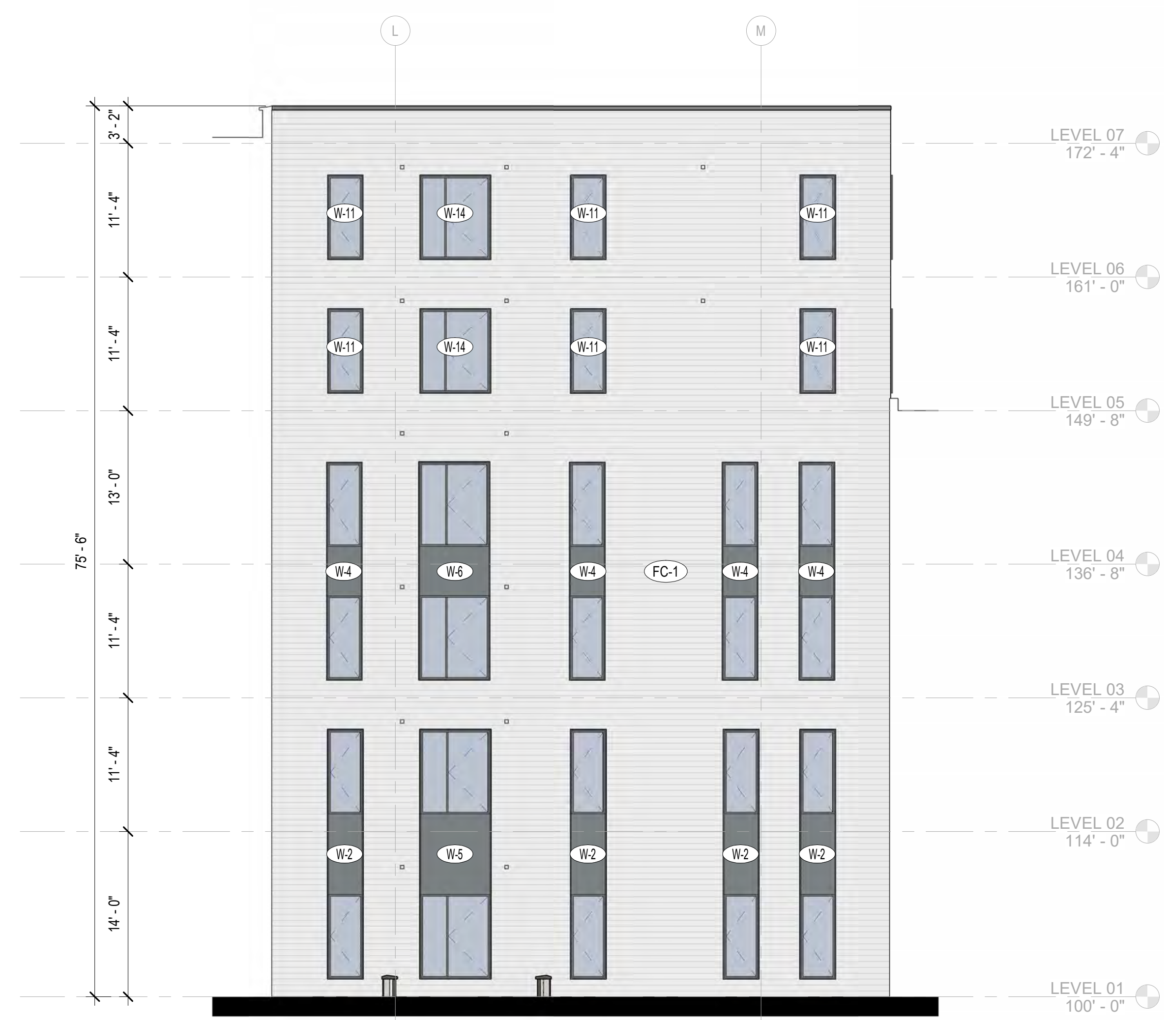
D3 ENLARGED ELEVATION - EAST - ENCLOSED A6.107 1/8" = 1'-0" 0' 4' 8' 16'
